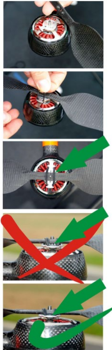
figure 25: mounting the rotor blades
