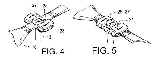
The written description further explains that "[t]he counterclockwise lock mechanism 11C operates in a similar fashion with an opposite spin direction." Ex. 2002 at [0034]; *see also* Ex. 2003 at 8:19-20. Accordingly, these figures provide additional support for the "partial counterclockwise rotation" and "partial clockwise rotation" limitations that appear in revised proposed claim 12 and 13, respectively.
