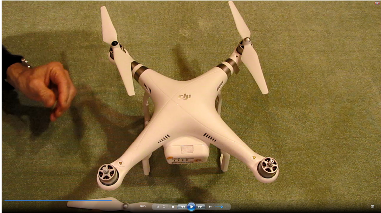
(Screenshot C): Video at 00:25: Clockwise Rotor Blade correctly installed
