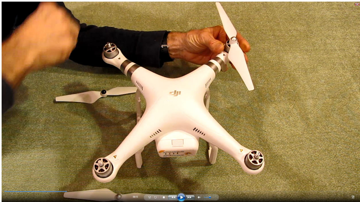
(Screenshot B): Video at 00:15: Counterclockwise Rotor Blade correctly installed
