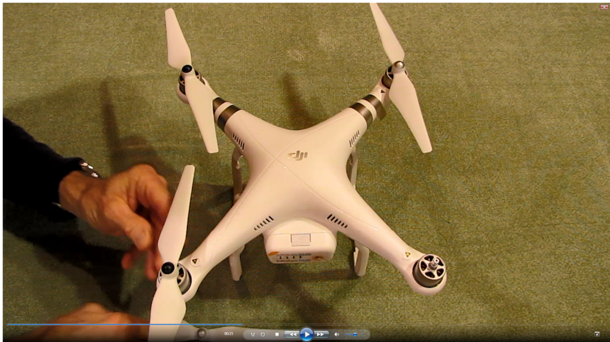
(Screenshot D): Video at 00:35: Clockwise Rotor Blade incorrectly installed on Counterclockwise shaft (black hub blade on silver tipped shaft)
