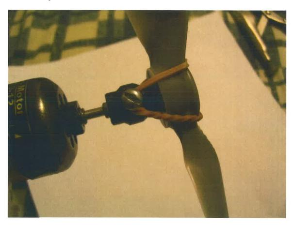
The prop sits on the tip of the yoke, swallowing it slightly. The rubber band holds it to the yoke and delivers the rotational force to the prop like a normal nut would, except with a bit more elasticity. That way, the prop's blades don't take the brunt of a crash, but rather the rubber band, as this picture shows:
