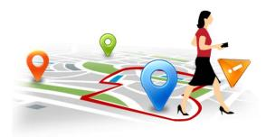
As seen above, a geo-fence alerts a user or system when a device enters or leaves the geo-fenced region. Because a geo-fence system has full knowledge of the geo-fence region it supports (*i.e.*, the region's defining line segments and arcs), and the position of a user's device is known from one of the techniques discussed above, an easy geometrical determination reflects whether that device is inside or outside a geo-fence.
