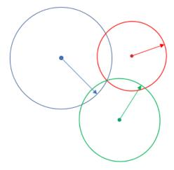
If we use distance information from two transmitters, the user's location is one of two intersections of the circles for those transmitters. For example, if we only use information from the blue and green transmitter, we can only resolve the user's position as reflecting two possibilities illustrated as the two intersections of the blue and green circles.
