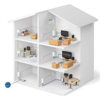
The range of powerline communication devices is limited, however, to within a building or sometimes to within a larger electrical circuit within a building. Similarly, telephone wire based communications can communicate data through existing telephone lines within a building.
