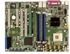
The new motherboard also leverages Intel's latest E7210 chipset. It's first single-processor chipset that boasts 64-bit functions, permitting standard inexpensive Pentium-4 microprocessors to be paired with high-bandwidth PCI-X slots.
