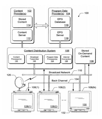
As shown, the system includes multiple content providers 102, which are defined as content sources, such as MSO cable television providers like "Comcast," as well as other non-MSO sources like "antenna, camcorders, VCRs, and digital camera." *Id.* at 2:56-60; 3:1-6. The content providers include stored content 114, such as "television programs," "live" content, and "movies," and content servers 112 for
