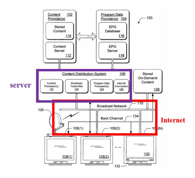
Specifically, content distribution system 106 may comprise software and hardware, including content processor 122, program data processor 124, broadcast transmitter 120, and an Internet connection 125. *E.g.*, *id.* at 9:29-31, 12:5-7 ("The method can be implemented in connection with any suitable hardware, software, firmware or combination thereof."). The software and hardware are for receiving and processing EPG data from program data provider 104, as well as video content,
