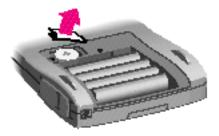
**5** Use a small screwdriver to pry the old backup battery out of its compartment.
