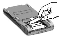
**5** Slide the battery compartment cover back on.
