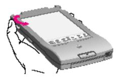
*Optional:* If you purchased the Newton power adapter, you can connect it to your MessagePad and plug it in to conserve battery power. The power adapter plugs into the port beneath the rubber flap marked with the — icon.
