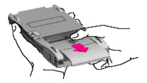
3 Install four AA batteries in the battery compartment. Make sure you position each battery's + and - terminals according to the diagram in the compartment (the batteries don't all have the same orientation). If you install the batteries wrong way, they may leak and damage your MessagePad. Leaking batteries may be hazardous.
