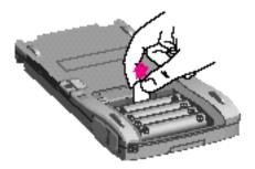
4 Insert four new AA batteries or a rechargeable battery pack, taking care to install them so they match the +/— polarity marked in the battery compartment. If you install the batteries the wrong way, they may leak and damage your MessagePad. Leaking batteries may be hazardous.
