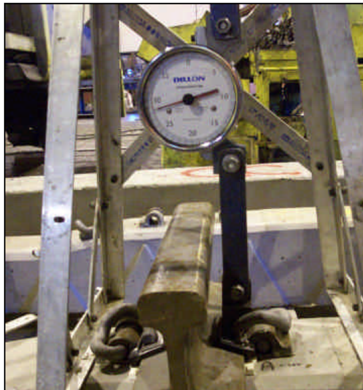
Figure 8 – Pandrol Toe Load Testing on CN 60E Tie
