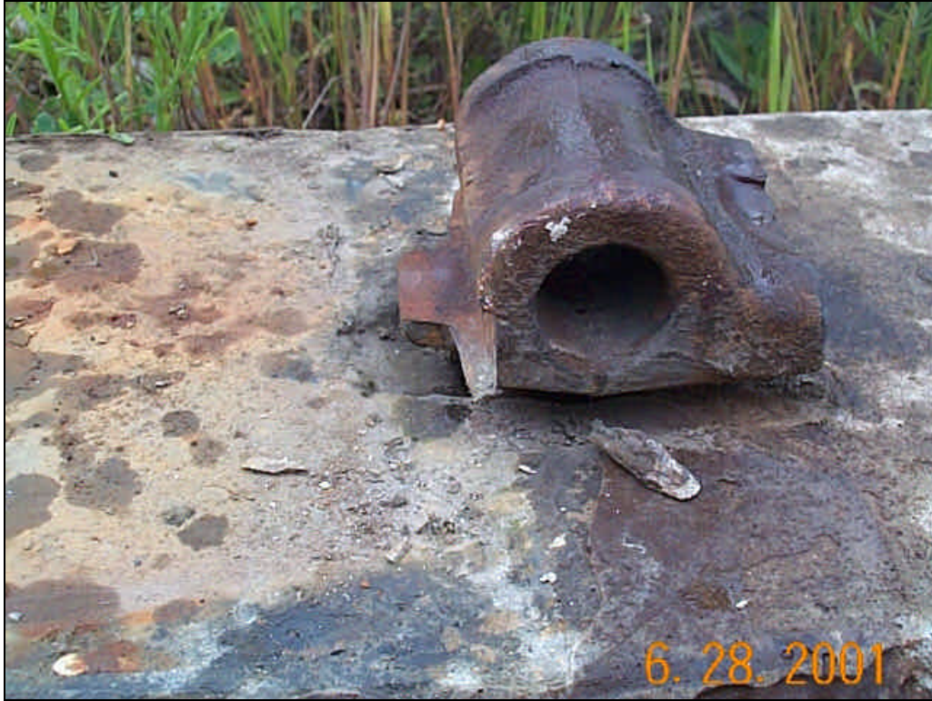
Figure 5 – Shoulder Showing Signs of Stem Fatigue, Heel Wear, and Face Wear
