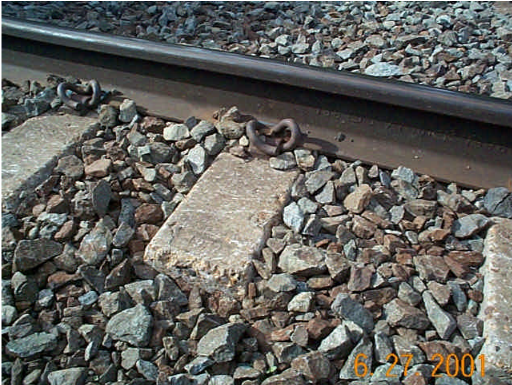
Figure 1 – Original 1972 CC241 (BR F23) Tie in Jasper Test Track
