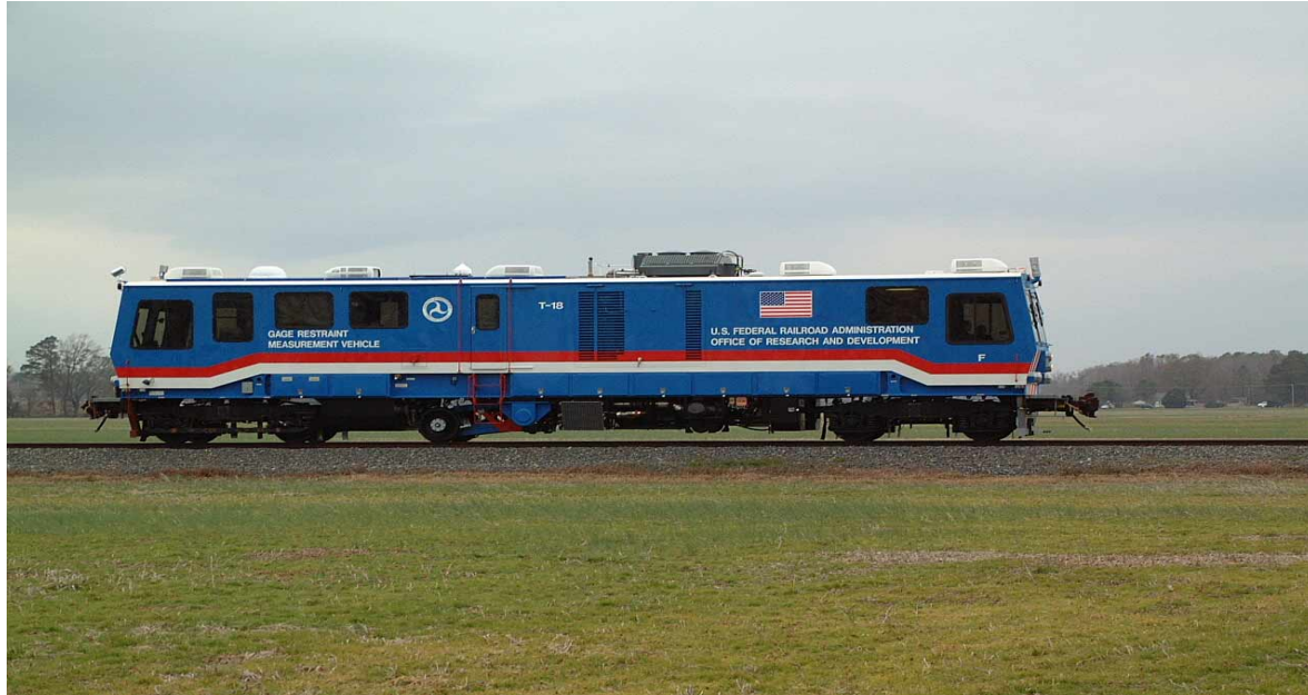
Figure 6. FRA T18 – Gage Restraint Measurement Car (GRMS)
