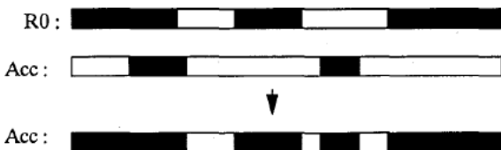
Figure 1.12, Point logic operation, OR between R0 and the accumulator
