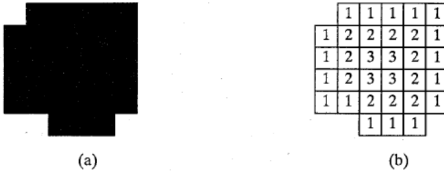
Figure 12.3. Distance transform of a binary object
