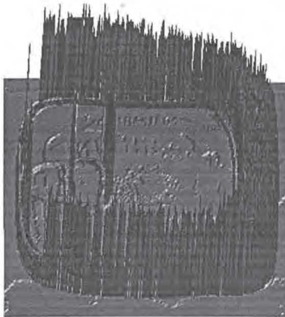
A3D plot of an unfiltered range image of a fish conserve can illustrating the effects of occlusion.
