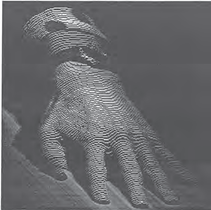
A 256x256 range image plotted as stacked height curves and with the intensity information as plot intensity.
