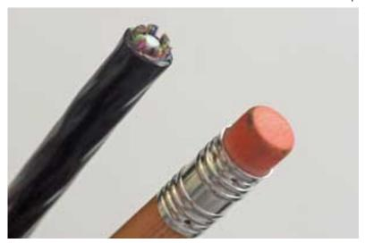
The other use for BI fibers is is make cables with as many fibers as possible. This has led to cables with 1728 fibers like this one from Prysmian as well as 3456 and 6912 fibers.
