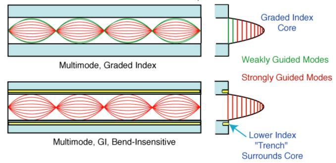
In regular graded index multimode fiber, there are many modes (or rays of light - about 400 of them) being transmitted down the fiber. The inner modes are "strongly guided" which means they have little sensitivity to bending stresses. But the outer modes are "weakly guided" which means they can be stripped out of the core when the fiber is bent.
