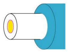
When you look at the end of a bend-insensitive fiber in a microscope with angled lighting, you can sometimes actually see the trench as a gray ring around the core.
