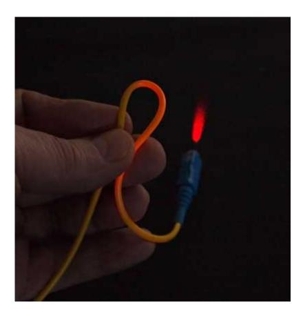
Fiber coatings and cables are designed to prevent as much bending loss as possible, but it's part of the nature of the fiber design. Bending losses are a function of the fiber type (SM or MM), fiber design (core diameter and NA), transmission wavelength (longer wavelengths are more sensitive to stress) and cable design.
