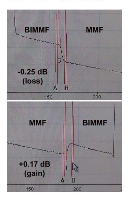
Another problem arises when testing mixes of BI MM and conventional fibers with an OTDR. Some BI fiber has a larger scattering coefficient than regular fibers and can create large
