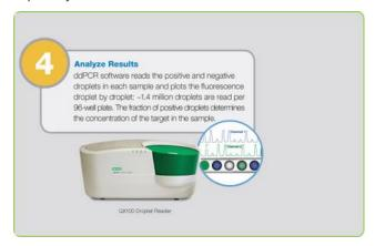
Positive droplets, containing at least one copy of the target, exhibit increased fluorescence over negative droplets. In ddPCR, the QuantaSoft software measures the numbers of droplets that are positive and negative for each fluorophore (for example, FAM and HEX) in a sample. The fraction of positive droplets is then fitted to a Poisson distribution to determine the absolute initial copy number of the target DNA molecule in the input reaction mixture in units of copies/µl.
