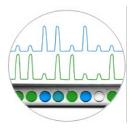
**Digital droplet reading.** Fluorescence measurements for each droplet in two optical channels are used to count the numbers of positive and negative droplets per sample.
