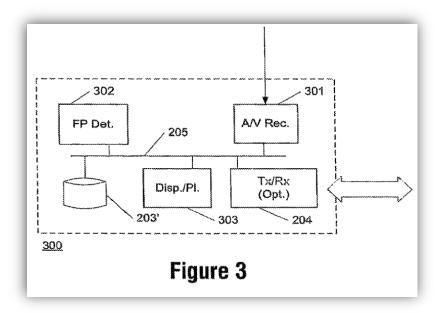
Referring to Figure 1b below, fingerprinting detector (302) receives the signal (101) from signal receiver (301) and generates a fingerprint stream (104). This stream is compared to the stored reference fingerprints (102) ('FP1', 'FP2', etc.) in database (203'):
