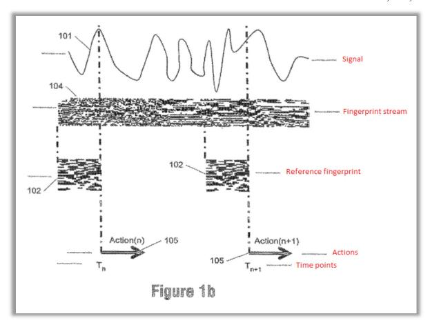
Ex-1001, Fig. 1b, 7:28-37. Like the process for generating fingerprints, matching fingerprints was already known in the art. Id., 6:25-42. When a match is found, the representation of the associated action (105) ('A1', 'A2', etc.) is retrieved and executed by the playback device at the associated time point ( $T_n$ ;  $T_{n+1}$ ). Id., 5:65-6:20, 7:36—40; Ex-1007 ¶47-48.
