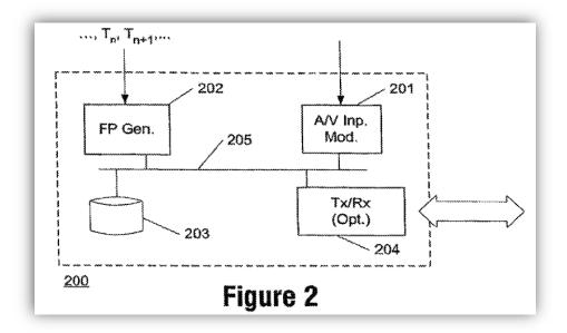
Ex-1001, Fig. 2, 6:48-58; Ex-1007 ¶¶ 40-41. These modules and components are controlled by microprocessors. *Id.* Signal input module (201) receives analog or digital content as signal (101), which is fed to fingerprinting module (202) to calculate fingerprints (102):
