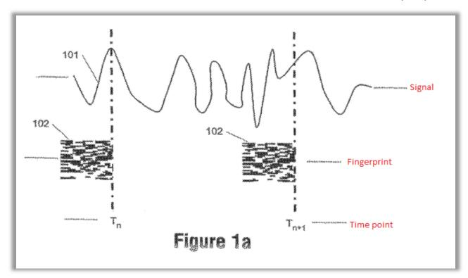
Ex-1001, Figs. 1a, 2, 3:50-52, 4:15-23, 6:59-64; Ex-1007 ¶¶42-43. Fingerprints are generated for each time point  $(T_n; T_{n+1})$  for which an action is to trigger during playback of signal 101. Ex-1001, 3:52-55, 4:15-17.
