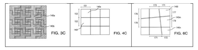
The specification discloses that the prior art electrodes have protruding digits that alternate with the adjacent electrodes to produce an "interdigitated" pattern as shown in Figures 3A-3C. *Id.* at 7:41-49 (describing interdigitated drive electrodes with respect to Figure 3A); *see also id.* at 7:57-8:3 (describing interdigitated sense electrodes with respect to Figure 3B).
