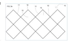
example, Figure 2a (to the right) is described as follows: "The electrode pattern 10 may be formed by a number of straight conductive lines 11 arranged to interconnect at connection points to define a conductive grid or mesh pattern made up of an array of square shaped mesh cells 13 arranged in a layer." '574 patent at 3:64-4:1.
