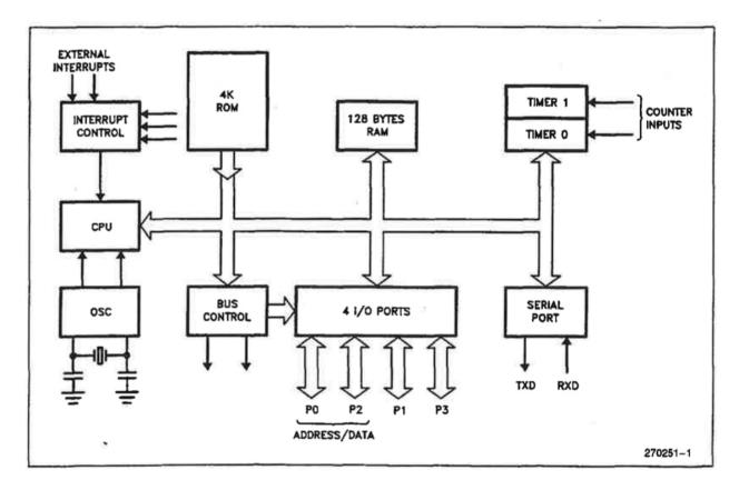
The 128 bytes of RAM comprise a stack pointer, 4 banks of 8 registers denoted as R0-R7, and a possible bit-addressable space (bit addresses 0-7F) as depicted in the
