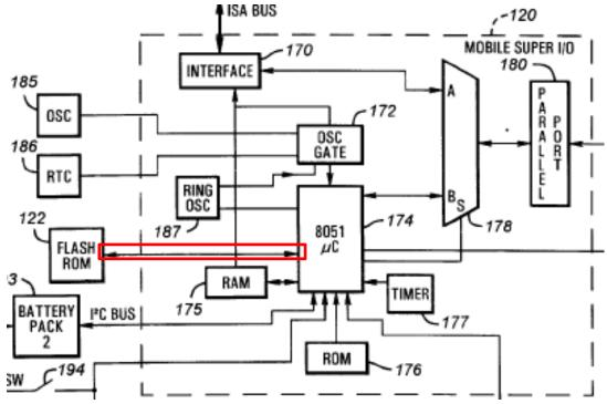
Le also discloses a microcontroller that fetches program instructions or data from the flash ROM. A POSITA would have understood that the bus transfers data between the flash ROM and the microcontroller because it is the only path for transferring data. Id.,  $\P$  62. Le teaches that the microcontroller can fetch the program instructions or data from the non-volatile memory via the non-volatile memory bus.
