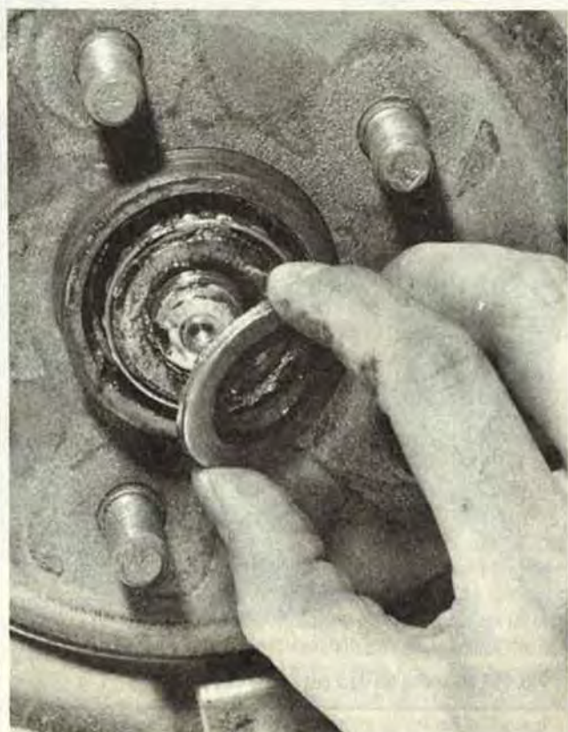
FIG. 55E Removing the washer — rear wheel bearings
