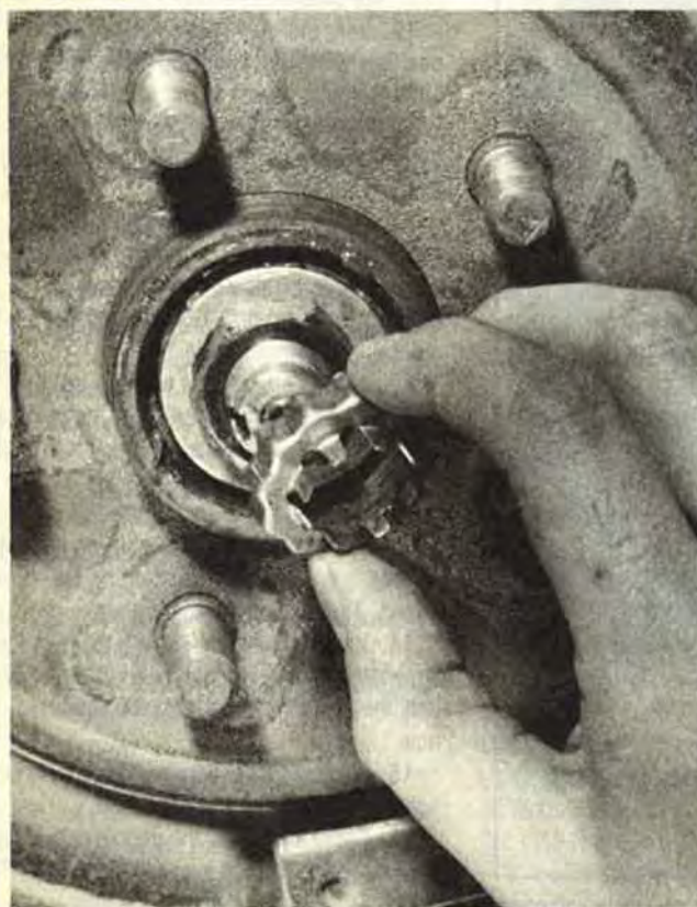
FIG. 55C Removing the locknut retainer — rear wheel bearings
