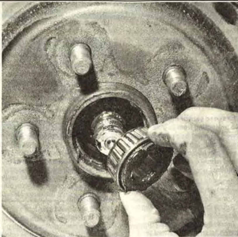
FIG. 55F Removing the rear wheel bearings
