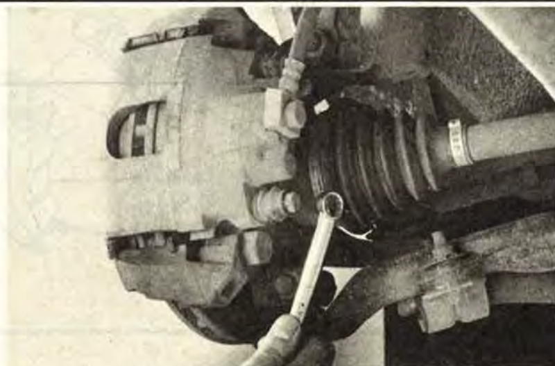
FIG. 24C Removing the front caliper
