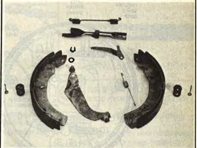
FIG. 52F Rear brake shoe hardware
