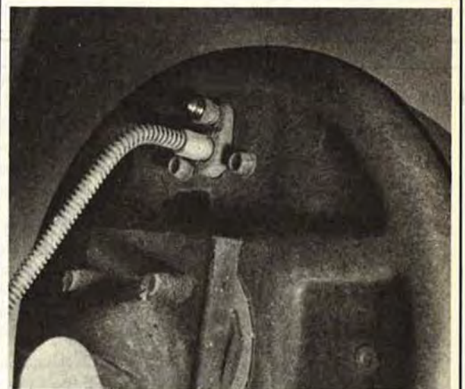
FIG. 52H Bleeding the rear brakes
