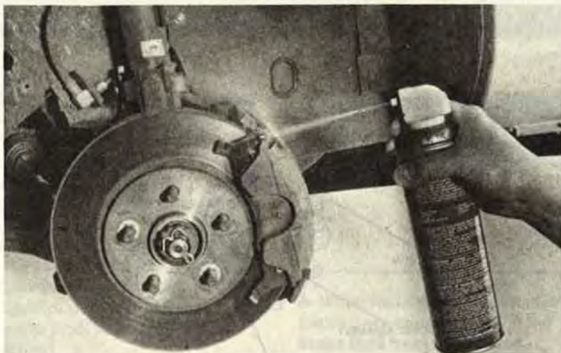
FIG. 24A Replacing front disc brake pads
