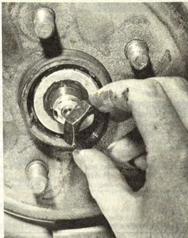
FIG. 55D Removing the locknut — rear wheel bearings
