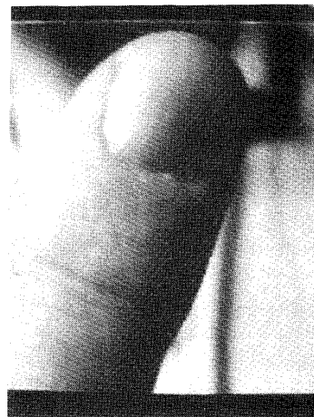
Figure 4 : Grey-scale image formed by 128×128 pixel prototype sensor.
