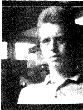
Figure 5 : Grey-scale image formed by 128 \times 128 pixel prototype sensor.
