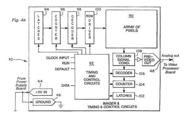
As shown in Figure 4a above, image sensor 40 contains array of pixels 90 and timing and control circuits 92. *Id.* at 12:40–42. Array of pixels 90 is an active pixel group and "[e]ach pixel circuit has its own amplifier which is controlled by the timing and control circuitry." *Id.* at 12:45–64.
