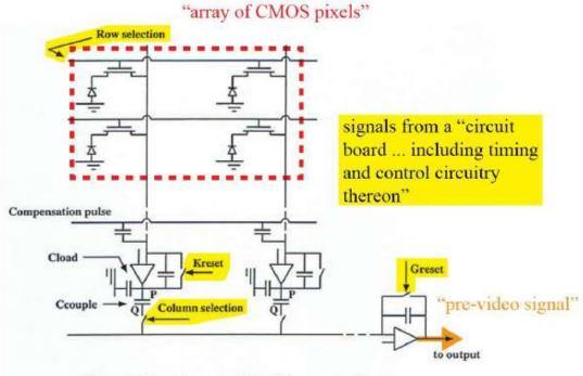
Figure 1: Schematic representation of the sensor architecture
