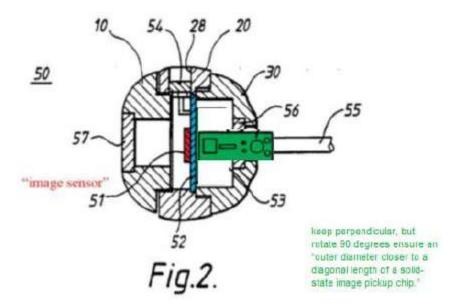
*Id.* at 64. The above annotated figure prepared by Patent Owner shows circuit board 53 perpendicular to circuit board 52, but rotated ninety degrees from what is shown in actual Figure 2. *Id.*
