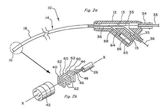
As shown in Figure 2b, an imaging device in the distal end 16 of endoscope 10 may include image sensor 40 electrically coupled, via pin connectors 62, to video processing board 50 and optional supplementary board 60. *Id.* at 9:58–10:8. Image sensor 40 may be bonded to lens system 42. *Id.* at 10:16–19.
