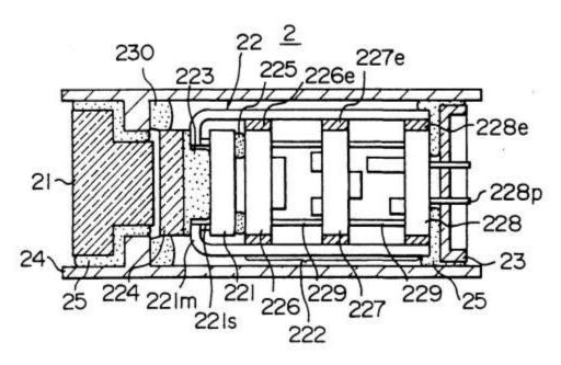
Figure 2 above shows camera head 2 with image pickup unit 22, the latter of which comprises solid-state image pickup chip 221 and circuit module 222. Ex. 1015, 2:38–41. Suzuki discloses the use of an 8.5 mm solid-state image pickup chip with an outer camera head diameter of about 10 mm. *Id.* at 4:6–11.
