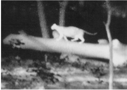
FIGURE 7.1 A thermal image of a house cat in a forested setting. The thermal signature of Sniper was captured with an InfraCAM® model A 3–5 \mu\text{m} infrared camera. The photo shown here was taken with a 35 mm camera of a single frame from 8 mm video of the thermal imagery displayed on a TV monitor.
