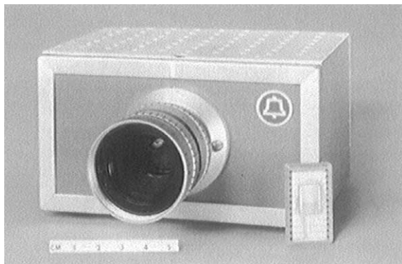
Fig. 10. A camera with all video circuitry contained in the box. The area imaging device shown had the 250 line resolution needed for the Picturephone application.
