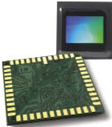
Aptina Imaging Corporation's 10-megapixel complementary metal-oxide semiconductor sensor is the first such device for point-and-shoot cameras.
