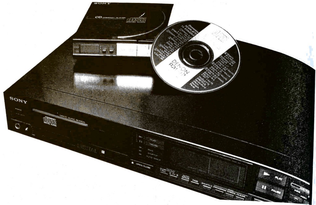
Figure 15-1. Sony D-5 in Comparison to Home-Size CD Player.
