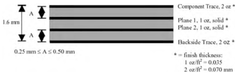
Fig. 7.8 Cross section of multilayer PCB in JEDEC standard
