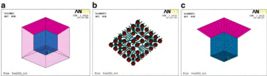
Fig. 8.27 FEA models of 40 pins MCSP for resistance and inductance: (a) Air and infinite volume (b) 40 bumps with RDL (c) partial mesh
