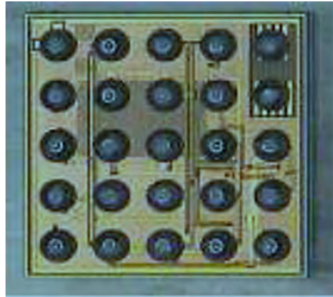
Fig. 6.6 The WLCSP for the power IC integration [4]
