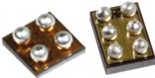
Fig. 6.3 Wafer-level chip-scale package for integration of Mosfet and protection/control IC
