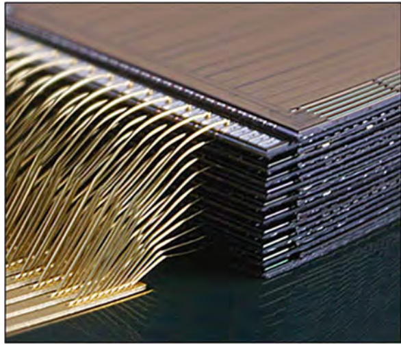
Fig. 4.4 1.4 mm MCP with 20 stacked dies ( source: Elpida Memory )
