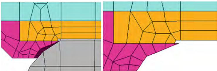
Fig. 10.43 Finite element model of copper UBM with 1 \mu\text{m} thick pocket
