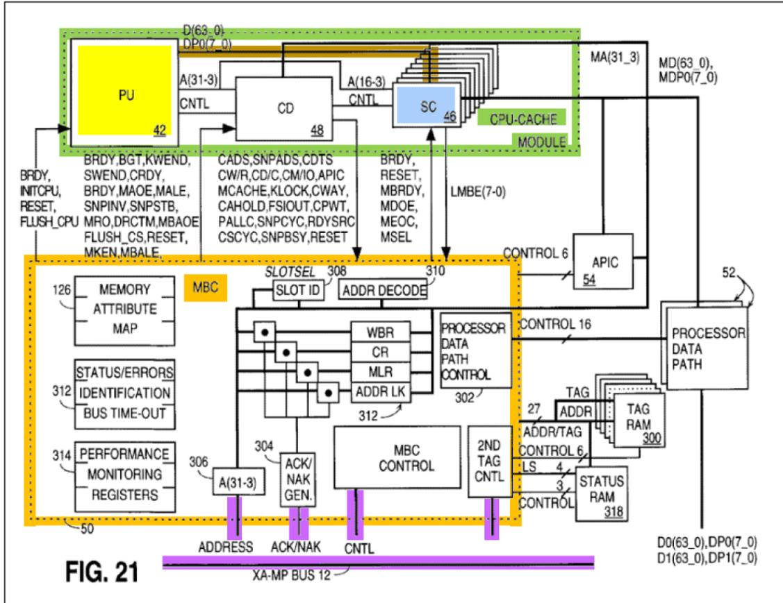
Pet. 88. Above is Petitioner’s annotated version of Wu’s Figure 21, a block diagram of a memory bus controller. See Ex. 1006, 2:32.
