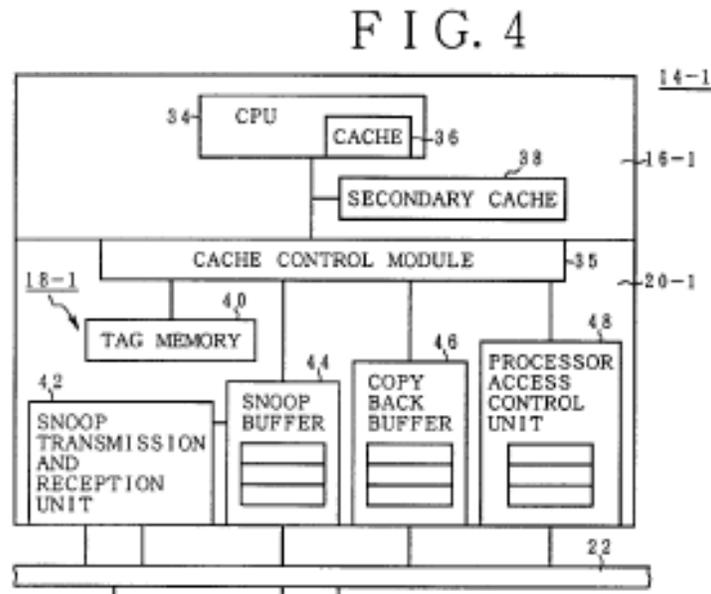
The figure above is a cropped version of Figure 4, which is a block diagram of an internal construction of the processor module of Figure 3. *Id.*
