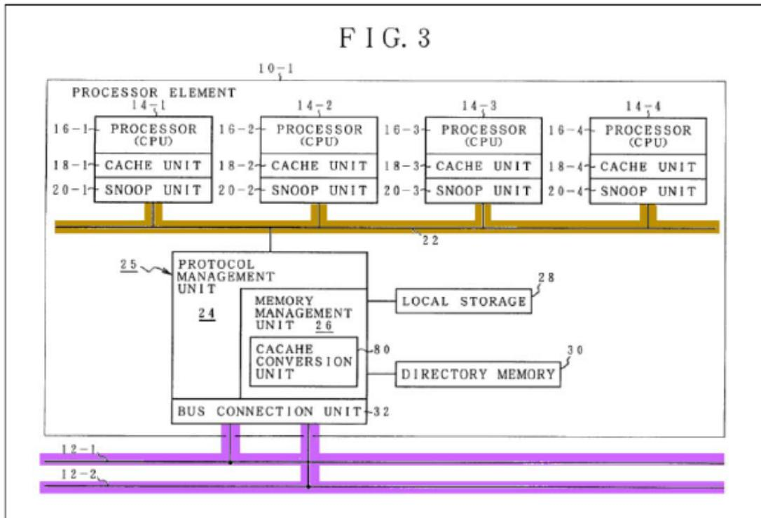
Above is Figure 3—a block diagram of an internal construction of a processor module—with, *inter alia*, Petitioner’s highlighting in gold of snoop bus 22. Pet. 51; Ex. 1005, 13:53–54. Petitioner contends that snoop bus 22 interconnects the four processors located in each of processor elements 14-1 through 14-4. Pet. 51. Petitioner continues:
