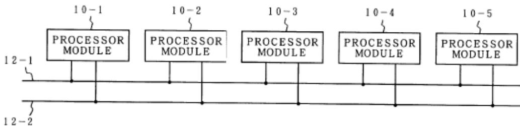
Figure 2 is a block diagram of a multiprocessor module construction of Kabemoto’s system. *Id.* at 13:51–52. Figure 2 depicts five processor modules, 10-1 through 10-5, connected via system buses 12-1 and 12-2. *Id.* at 16:8–14. Figure 3 is reproduced below.
