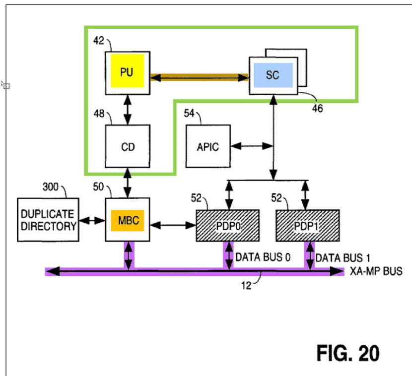
Pet. 87. The annotated figure above is Figure 20 of Wu, a block diagram of a processor functional unit, with a green line added to identify that which Petitioner contends is the claimed “processing system.” *Id.* at 68; Ex. 1006, 2:31. Petitioner contends that a plurality of “data paths” is shown in gold in the figure above. *See* Pet. 86.
