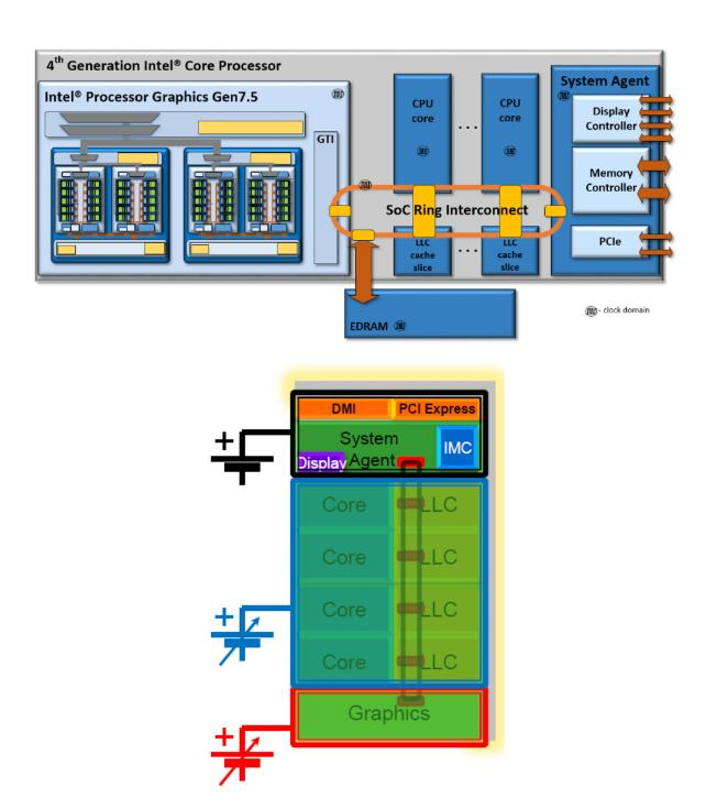
"wherein for at least some of the data processing units, the clock frequency is adjustable at runtime without affecting the clock frequency of at least one of: one other of the data processing units, and the bus system; and"
