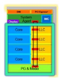
"each of the plurality of same level cache nodes is communicatively connectable with each of the plurality of processor cores via the bus system for transferring data between the respective cache node and respective processor core"
