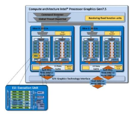
"a multi-level cache for caching instructions and data, at least one level of the multi-level cache comprising a plurality of cache slices, the multi-level cache being shared by the data processor core and the array data processor"
