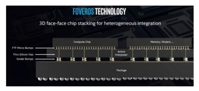
"at least parts of the interconnect structure are implemented on at least a second one of the at least two dies."
