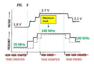
Pet., 41 (Nicol's Figure 3 as annotated by Petitioner). If Kling's voltage limit is below 2.7 V, the 140 MHz "maximum frequency" will not be reached. If Kling's voltage limit equals 2.7 V, the power consumption will be dropped immediately after the "task started," and Petitioner presents no evidence that the overtemperature threshold would be reached. Therefore, Petitioner fails to prove a reasonable expectation of success in achieving the claimed method by combining
