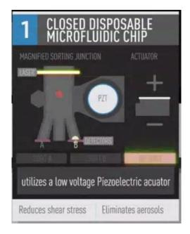
44. Inspection of a WOLF Cell Sorter product further shows that the WOLF Cell Sorter includes actuator and "buffer" reservoirs to generate and absorb pressure pulses for sorting particles, as shown in the photograph below. A flexible membrane covers at least a portion of the chip, including above the buffer reservoir. This flexible membrane absorbs the pressure pulse generated by the actuator.
