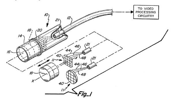
Figure 1 is an enlarged fragmentary partially exploded perspective view of the distal end of a camera module used in conjunction with a PDA. *Id.* at 7,
