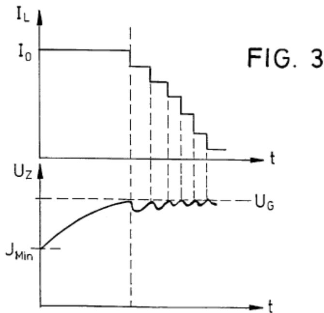
Figure 3 of Baumann depicts two graphs showing the relationship between charge current  $I_L$  over time, and battery voltage  $U_Z$  over time. See Ex. 1007, 4:63–5:35. As shown in Figure 3, after the voltage  $U_Z$  hits a
