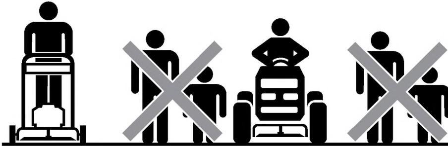
Ref ANSI B71.1 2003 (derived from ISO 11684 Figure B.2.6 and section D.9 – communicating idea of prohibited action or hazardous location)
