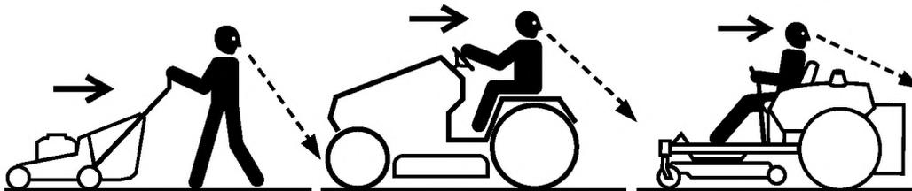
Ref: Derived from ISO 11684 section D.8 "Using arrows to show visual elements and machine motion."
