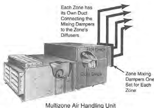
Figure 24.1 Multizone Dampers
