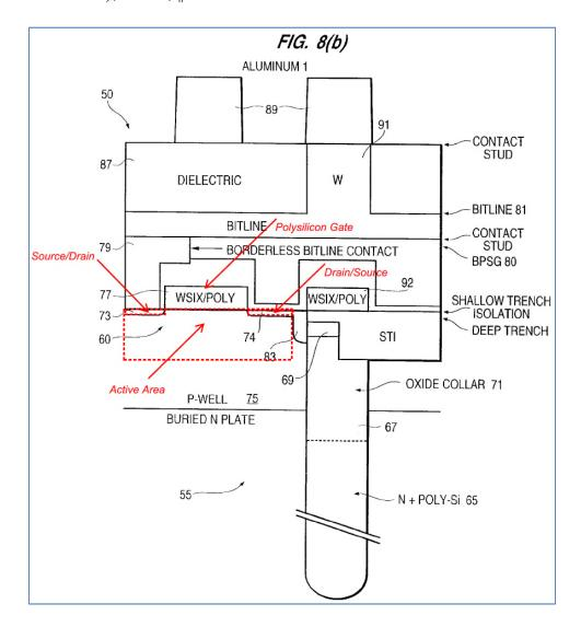
Similarly, Saki teaches the formation of source/drain regions in connection with "a method of manufacturing the DRAM cell 50 using the shallow isolation
