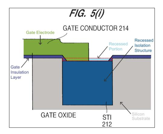
(iv) [1.3] "a gate electrode and a gate insulation layer formed above said substrate, a portion of said gate electrode and said gate insulation layer extending into said recess above said recessed isolation structure; and" and [13.3] "a gate electrode comprised of polysilicon . . "
