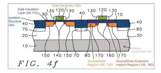
Lu discloses that the "thinner" gate oxide 90 has a thickness of 30 to 60 Å, the "thicker" gate oxide 110 has a thickness of 50 to 80 Å, and the polysilicon gate electrode 120 has a thickness of 0.1 to 0.4  $\mu$ m, which is equivalent to 1000 to 4000
