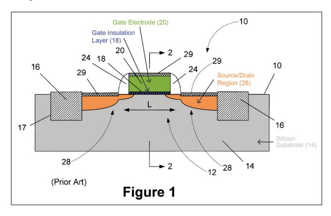
Specifically, a transistor (element 10) is formed in and on a silicon substrate (element 14) and has four terminals: a gate electrode (element 20) that is isolated from the substrate (element 14) by a gate insulation layer (element 18), and source
