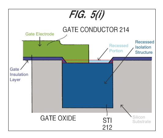
(iv) [23.3] "a gate insulation layer and a gate electrode positioned above a portion of said upper surface and a portion of said exposed sidewall surface of said active area; and"
