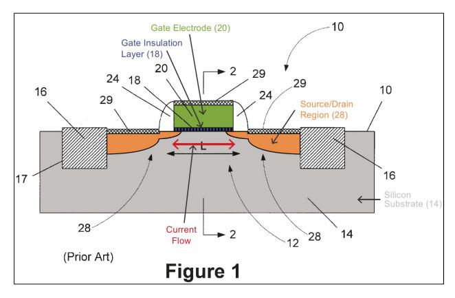
The source and drain are doped areas (active regions) that are the sources for particles (e.g., electrons or holes) to flow into and out of the channel. Kiaei,  $\P$ 49. The channel region is lightly doped with a dopant type that is opposite to that of the source and drain. *Id.*
