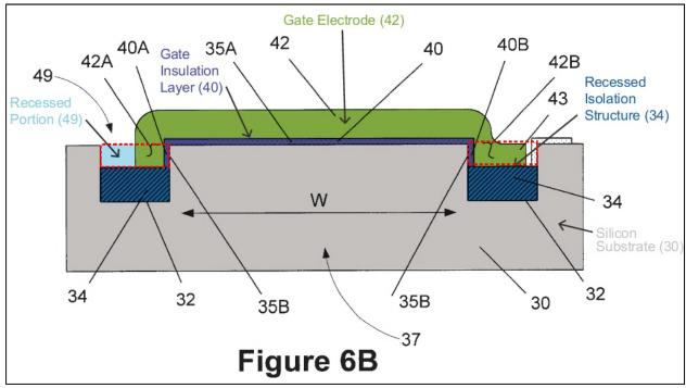
The transistor includes substrate 30 with gate electrode 42 and gate insulation layer 40 formed on the substrate. Ex. 1001, 6:62 – 7:3; Kiaei, \$\mathbb{P}62\$.
