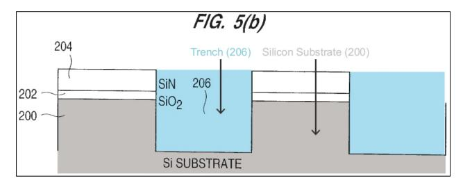
(iii) [1.2] and [13.2] "a recessed isolation structure formed in said substrate, said isolation structure defining a recess thereabove;"
