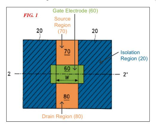
A POSITA, reading Yun, would recognize that conventional source and drain regions are formed in the active area over the substrate. Kiaei, \$\mathbb{P}99\$. For example, Fig. 1 of the '122 patent shows an "illustrative *prior art transistor* in the transistor length direction" ('122 patent, 3:9-10); as shown in the annotated figure
