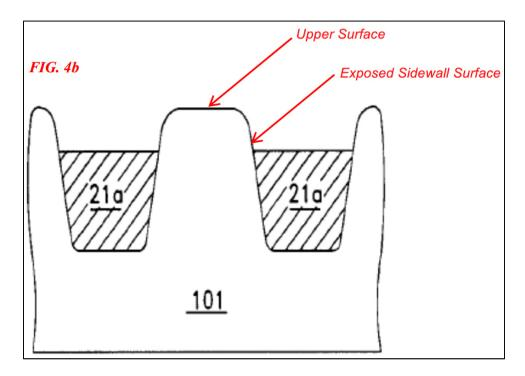
(iv) [23.3] "a gate insulation layer and a gate electrode positioned above a portion of said upper surface and a portion of said exposed sidewall surface of said active area; and"
