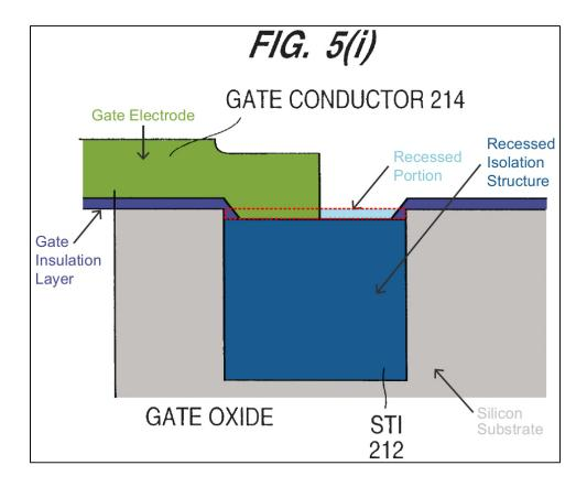
179. With respect to claim 13, I note that Saki teaches forming the gate electrode from polysilicon. For example, Saki teaches—in connection with "a method of manufacturing the DRAM cell 50 using the shallow isolation structure and method of the present invention"—forming conductive material (such as a gate electrode) using "N+-type polycrystalline silicon" or "undoped polycrystalline silicon." Saki discusses in detail its method of manufacturing DRAM cell 50 at 7:19-59.
