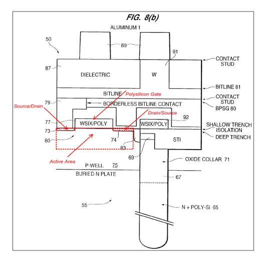
182. Similarly, Saki teaches the formation of source/drain regions in connection with "a method of manufacturing the DRAM cell 50 using the shallow isolation structure and method of the present invention." Ex. 1006 (Saki), 7:19-22. Saki specifically describes: "Using the gate electrodes as masks, *source/drain* regions may be formed by ion implantation." Ex. 1006 (Saki), 8:55-58.
