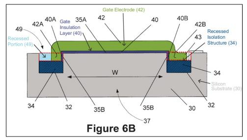
61. It is common to provide multiple views of a transistor to highlight different features; typical views include a top or plan view, along the length (L) dimension, along the width (W) dimension, and so forth. Certain transistor elements may be depicted in one view but not another. For example, the source/drain regions appear in the '122 patent's length dimension view (Fig. 7A above) but not in the width dimension view (Fig. 6B above).
