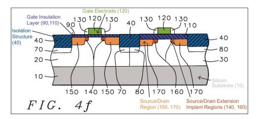
129. Lu discloses that the "thinner" gate oxide 90 has a thickness of 30 to 60 Å, the "thicker" gate oxide 110 has a thickness of 50 to 80 Å, and the polysilicon gate electrode 120 has a thickness of 0.1 to 0.4 μm, which is equivalent to 1000 to 4000 Å. Ex. 1005 (Lu), 7:2-13. With respect to the gate oxide thickness, Lu further explains that:
