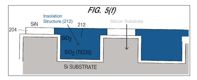
176. A series of etching processes are then carried out to remove portions of the pad silicon nitride 204 (*see* Fig. 5(g)), the pad silicon dioxide 202 (*see* Fig. 5(h)) and other "extensions" of the STI structure. Ex. 1006 (Saki), 4:59 – 5:7. The resultant transistor and isolation structure is shown in Fig. 5(i). I note, as shown in Fig. 5(i), that Saki's isolation structure defines a recess in the region above the silicon dioxide isolation structure, as indicated by the red dashed lines.
