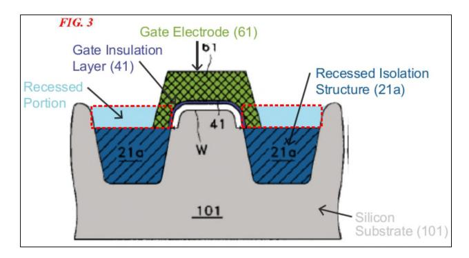
73. Yun's Figs. 4a and 4b (reproduced below), which provide views of the transistor fabrication process, further illustrate the formation of the recessed isolation region. Fig. 4a describes forming isolation region 21a using a "conventional trench isolation process." Ex. 1003 (Yun), 2-5. And in Fig. 4b, the oxide film in the trench is etched in order to increase the channel width, thereby forming the recess above. As Yun explains:
