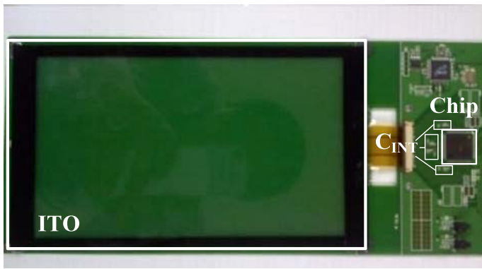
Fig. 8 Measurement board of sensor chip and ITO layer
