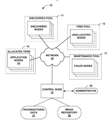
Figure 1 depicts distributed computing system 10 constructed from a collection of computing nodes. *See* Ex. 1001, 2:40–41, 3:54–56. Distributed computing system 10 includes physical computing devices or nodes operating in cooperation with each other to provide distributed processing, at least one control node 12, and network 18 that permits internode communications. *See id.* at 3:56–58, 3:62–66, 4:60–5:4. Control node 12 maintains organizational data 21, stores software image instances in
