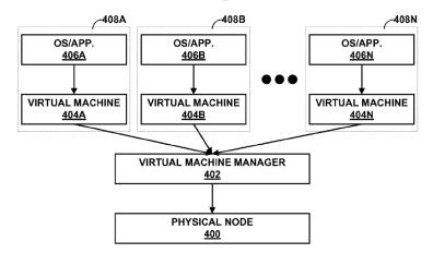
Figure 24 depicts a block diagram of a physical node to which a virtual machine manager and one or more virtual machines are deployed. *See* Ex. 1001, 3:28–30, 32:54–55. Physical node 400 may be any node within distributed computing system 10, for example, any one of application nodes 14. *See id.* at 32:56–58. Virtual machine manager 402 executes on
