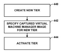
Figure 27A depicts a flow chart illustrating a procedure for autonomic deployment of a virtual machine manager to a node within the distributed computing system. *See* Ex. 1001, 3:38–40, 35:25–27. An administrator will create a new tier in step 440. *See id.* at 35:27–28. The administrator then specifies one or more captured virtual machine manager image instances for
