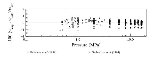
Figure 17. Comparisons of the speed of sound in the liquid phase calculated with the mixture model to experimental data for the R-134a/152a binary mixture.
