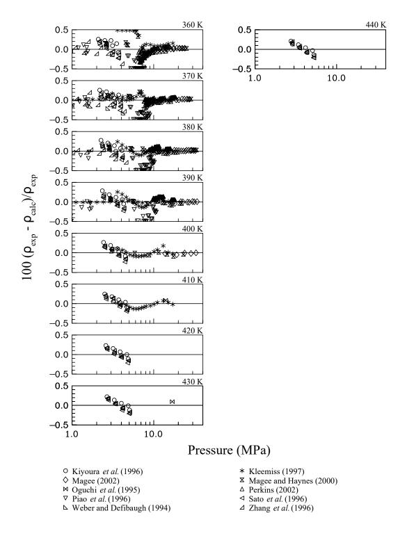
Figure 1. Comparisons of densities calculated with the mixture model to experimental data for the R-32/125 binary mixture (continued)
