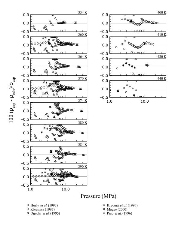
Figure 10. Comparisons of densities calculated with the mixture model to experimental data for the R-32/125/134a ternary mixture (continued).
