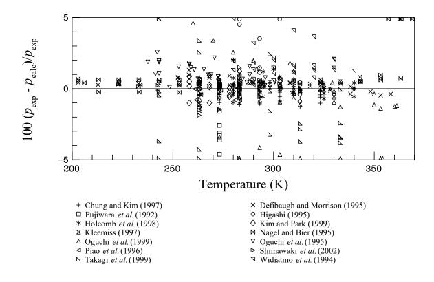
Figure 4. Comparisons of bubble point pressures calculated with the mixture model to experimental data for the R-32/134a binary mixture.
