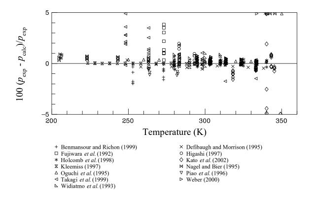
Figure 2. Comparisons of bubble point pressures calculated with the mixture model to experimental data for the R-32/125 binary mixture.
