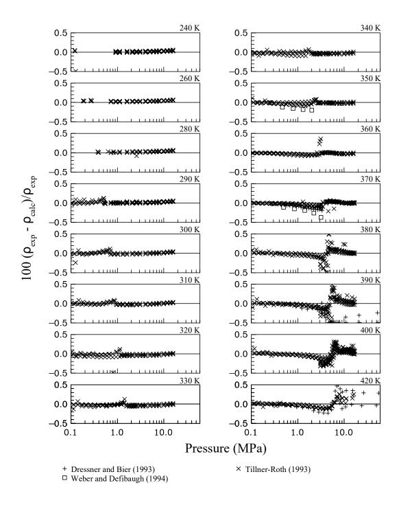
Figure 8. Comparisons of densities calculated with the mixture model to experimental data for the R-134a/152a binary mixture.
