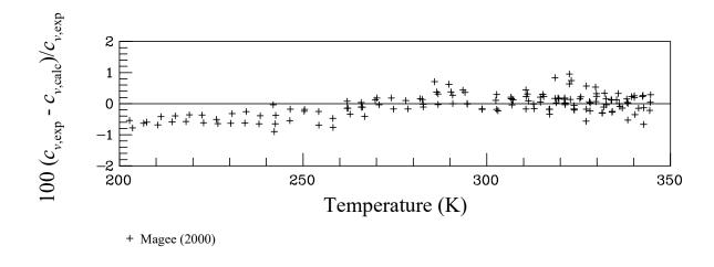
Figure 14. Comparisons of isochoric heat capacities calculated with the mixture model to experimental data for the R-32/125/134a ternary mixture.
