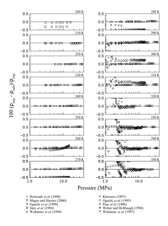
Figure 3. Comparisons of densities calculated with the mixture model to experimental data for the R-32/134a binary mixture.
