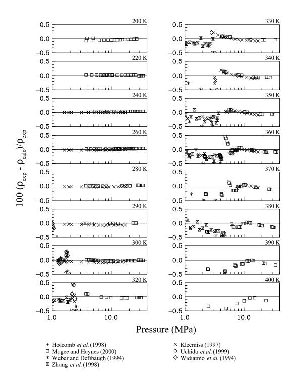
Figure 6. Comparisons of densities calculated with the mixture model to experimental data for the R-125/143a binary mixture.
