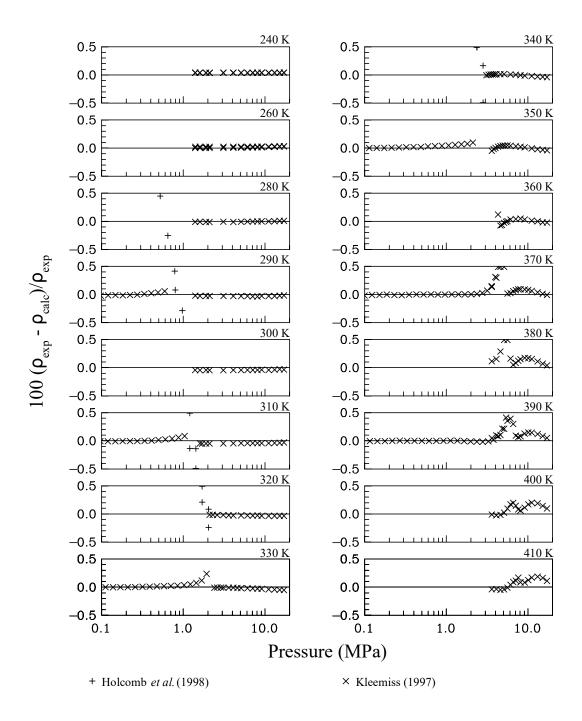
Figure 7. Comparisons of densities calculated with the mixture model to experimental data for the R-134a/143a binary mixture.
