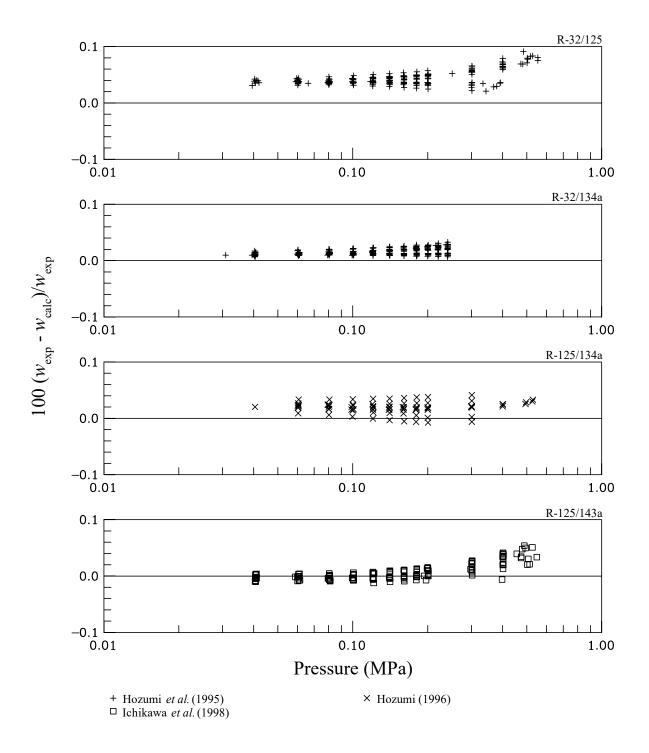
Figure 15. Comparisons of the speed of sound in the vapor phase calculated with the mixture model to experimental data for the R-32/125, R-32/134a, R-125/134a, and R-125/143a binary mixtures.
