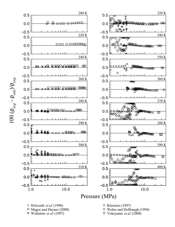
Figure 5. Comparisons of densities calculated with the mixture model to experimental data for the R-125/134a binary mixture.
