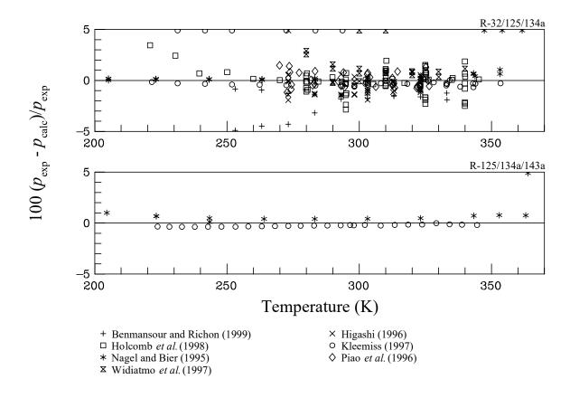
Figure 11. Comparisons of bubble point pressures calculated with the mixture model to experimental data for the R-32/125/134a and R-125/134a/143a ternary mixtures.
