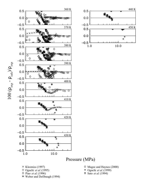
Figure 3. Comparisons of densities calculated with the mixture model to experimental data for the R-32/134a binary mixture (continued).
