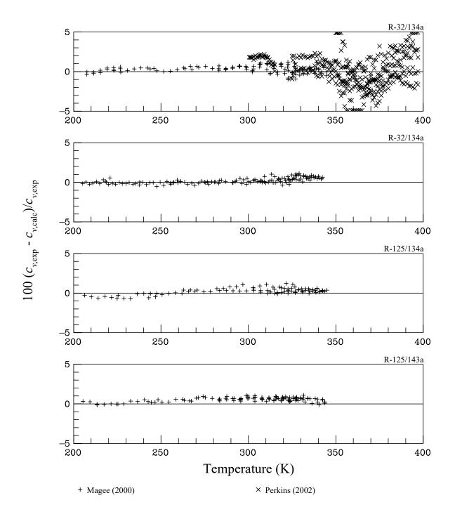
Figure 13. Comparisons of isochoric heat capacities calculated with the mixture model to experimental data for the R-32/125, R-32/134a, R-125/134a, and R-125/143a binary mixtures.
