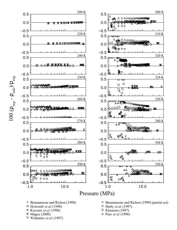
Figure 10. Comparisons of densities calculated with the mixture model to experimental data for the R-32/125/134a ternary mixture.
