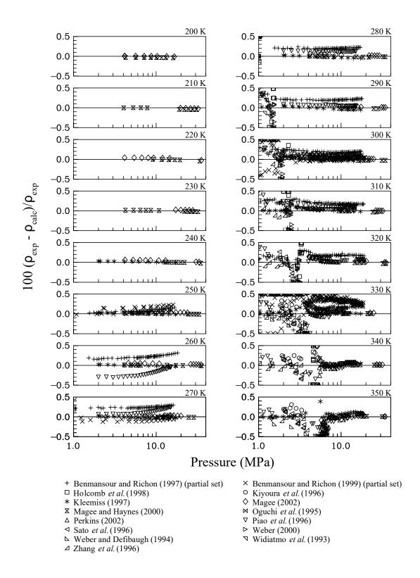
Figure 1. Comparisons of densities calculated with the mixture model to experimental data for the R-32/125 binary mixture.
