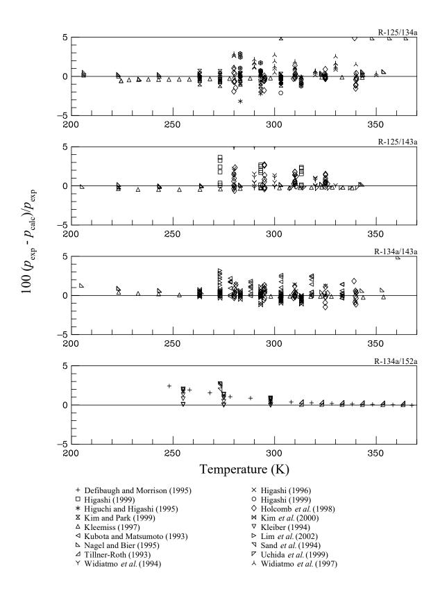
Figure 9. Comparisons of bubble point pressures calculated with the mixture model to experimental data for the R-125/134a, R-125/143a, R-134a/143a, and R-134a/152a binary mixtures.
