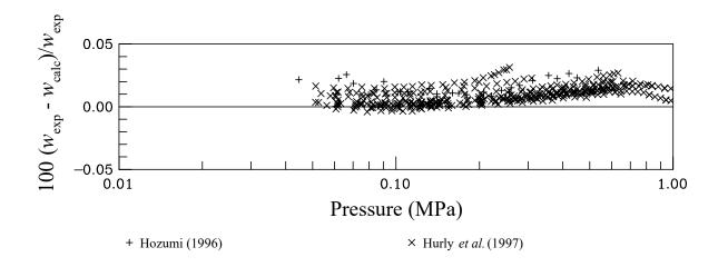
Figure 16. Comparisons of the speed of sound in the vapor phase calculated with the mixture model to experimental data for the R-32/125/134a ternary mixture.
