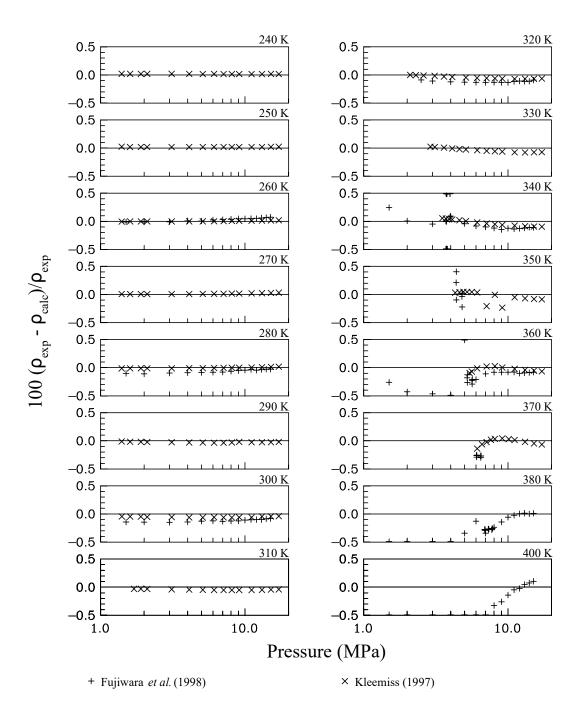
Figure 12. Comparisons of densities calculated with the mixture model to experimental data for the R-125/134a/143a ternary mixture.
