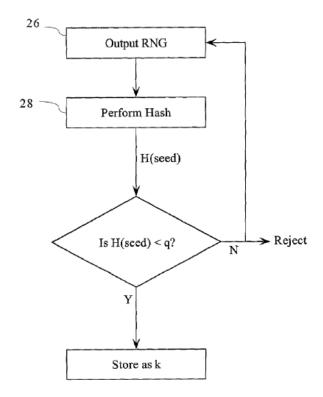
Figure 2 is a flow chart depicting the method for generation of ephemeral private key k disclosed by the '961 patent. *Id.* at 3:12–13. As shown in Figure 2, the method begins by obtaining a seed value from a random number generator, and then performs a hash function on that seed value to produce an output H(seed). *Id.* at 3:64–4:10. To eliminate the potential bias in the selection of k observed in DSS, the '961 patent discloses that
