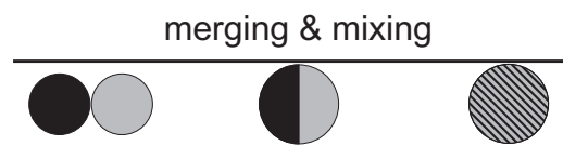
Figure 31. Schematic of reaction initiation by merging and mixing two drops.
