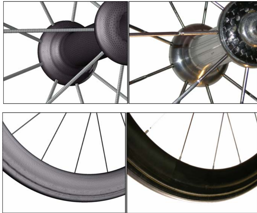
Figure 4. Mesh near hub (top) and wheel (bottom) compared to the actual Zipp 404 wheel
