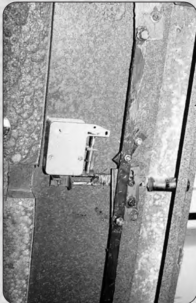
6. Properly functioning arrangement. Both rectangular pivot bars are vertical pulling the bolts into the safe door (top and middle bolts).
