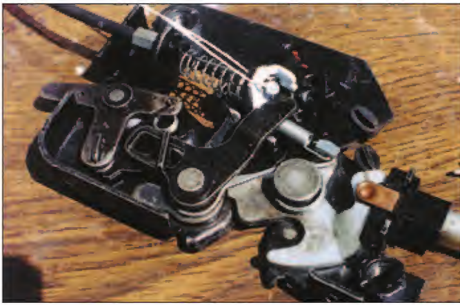
6. Wrap the wire around the cable connection.
