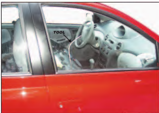
7. Lower the tool into the front passenger door.
