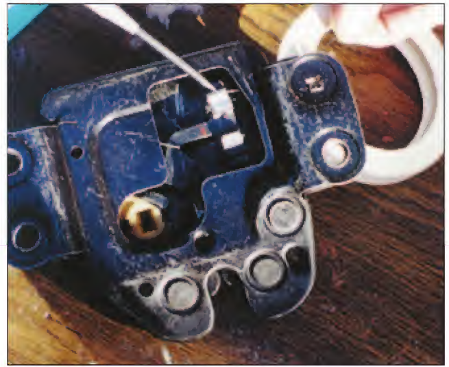
4. Wrap the wire around the release lever.
