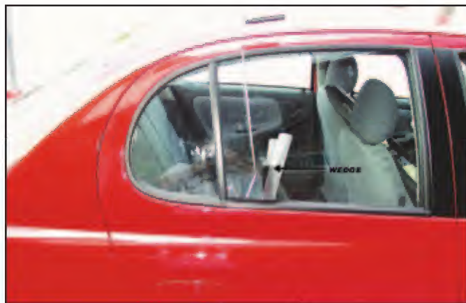
2. The tool is inserted at the rear door.
