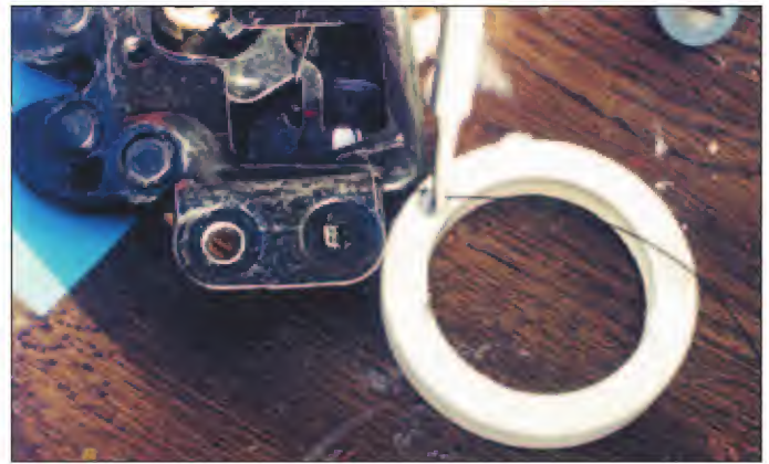
8. Wrap the wire around the Quick-Out screw.
