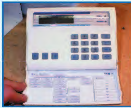
14. Alarm style keypad with a backbit 2 line LCD display.
