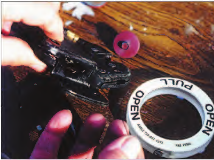
3. Fish the wire through any latch opening.
