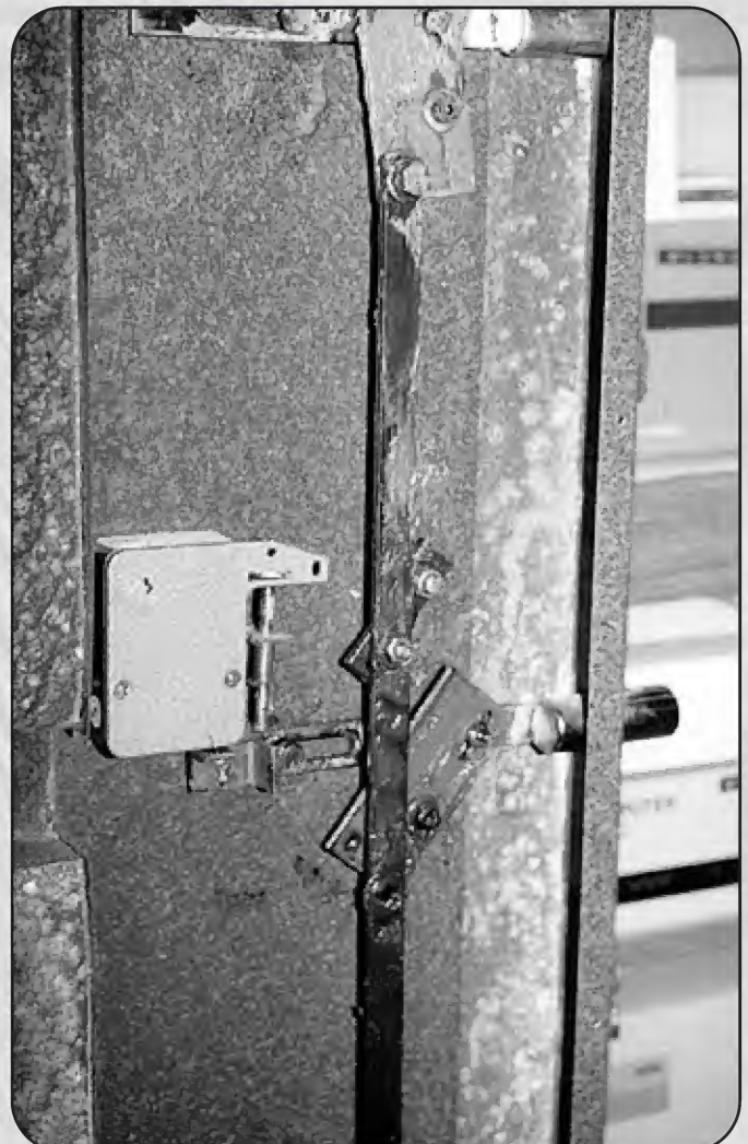
7. Center pivot unbolted. Top bolt is withdrawn while center bolt is still locked. Note positions of rectangular pivots.
