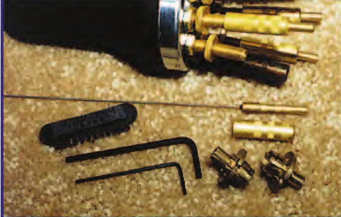
3. This photo shows the Allen wrenches, decoder bar and other available tips for the tool.
