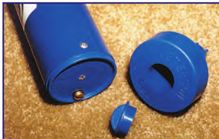
2. The cylinder of PVC has a specially built holder that is held into the tub by rivets. The holder fits the tool snugly while the cylinder cap houses the accessories.
