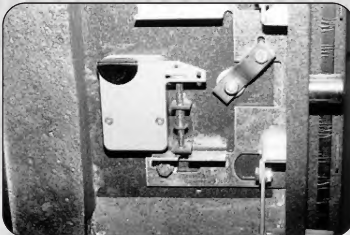
2. Inside bolt work of the small unit. Note relock cover on S&G lock.
