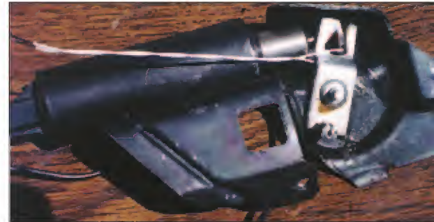
5. Wrap the wire around the solenoid lever.
