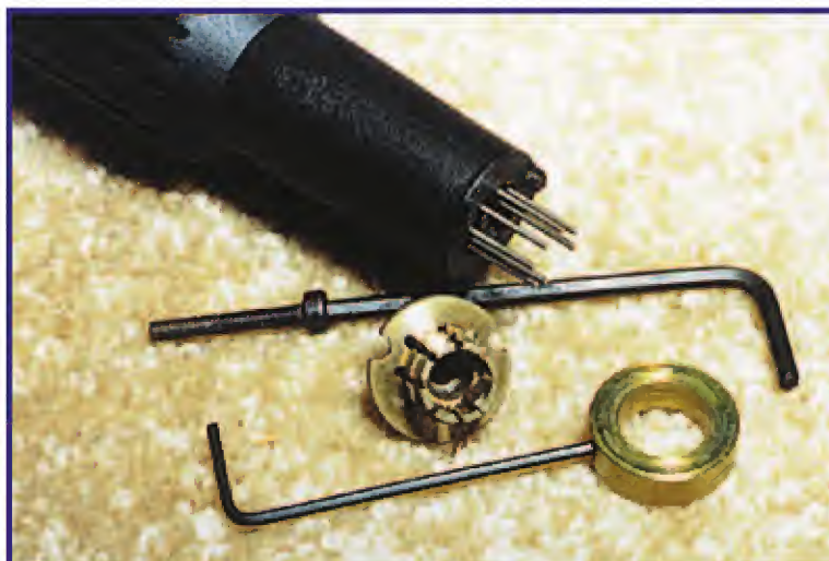
5. Here the tip is removed with the Allen wrenches in their perspective screws. The tip, which is anchored to the tool by the long Allen screw down its center, is seen with two notches on its outer rim.
