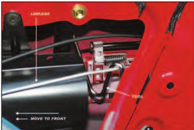
6. Move linkage to the front of the vehicle.
