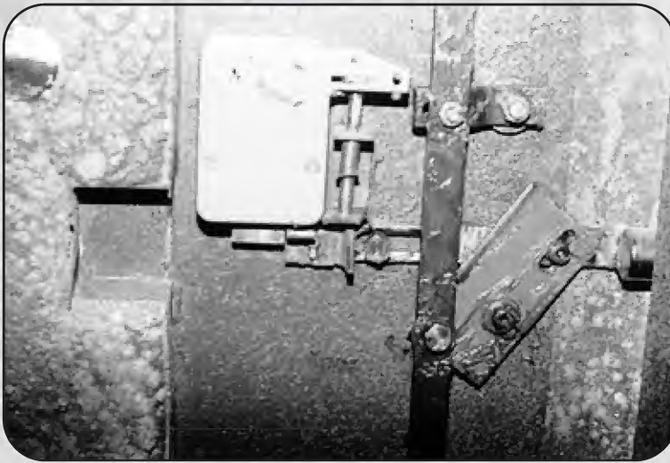
5. Bolt arrangement on Liberty Safe. Bolt bar and bolts move in different directions.
