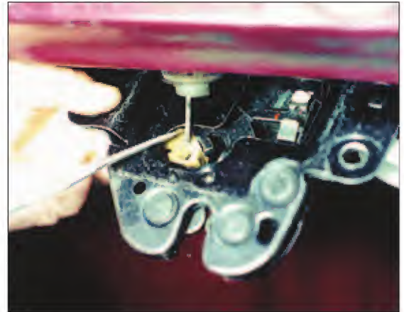
9. Reinstall the lock mechanism.
