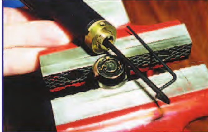
4. The standard tip has been installed and is being tightened by the Allen wrench through its center.
