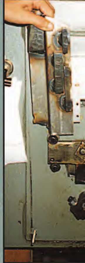
3. (below, right) The boltbar welded back together.
