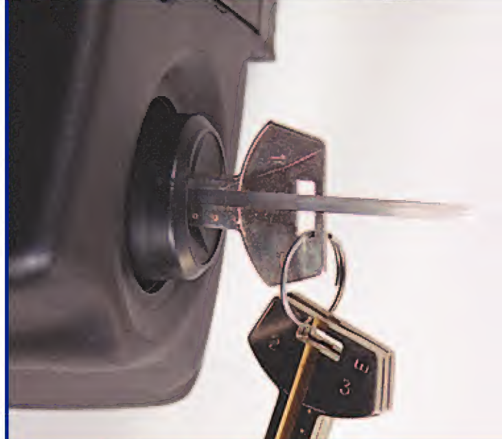
22. Insert key #1 up to the #4 Position Index mark using the Wafer Slide to lift and bypass wafer position #2.
