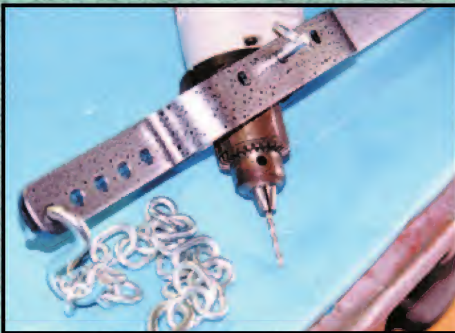
19. Drill rig with chain and spacer holes at end of rig.
