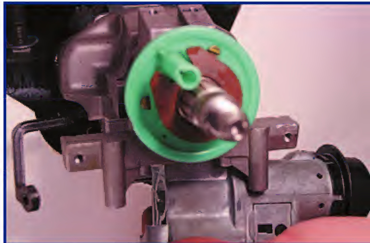
15. Remove the old lock and reinstall a new lock.
