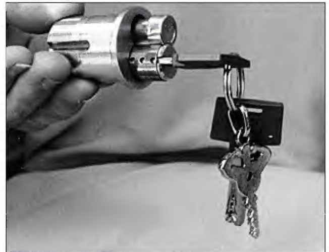
2. The IC lock as it is being taken out of the lock housing.
