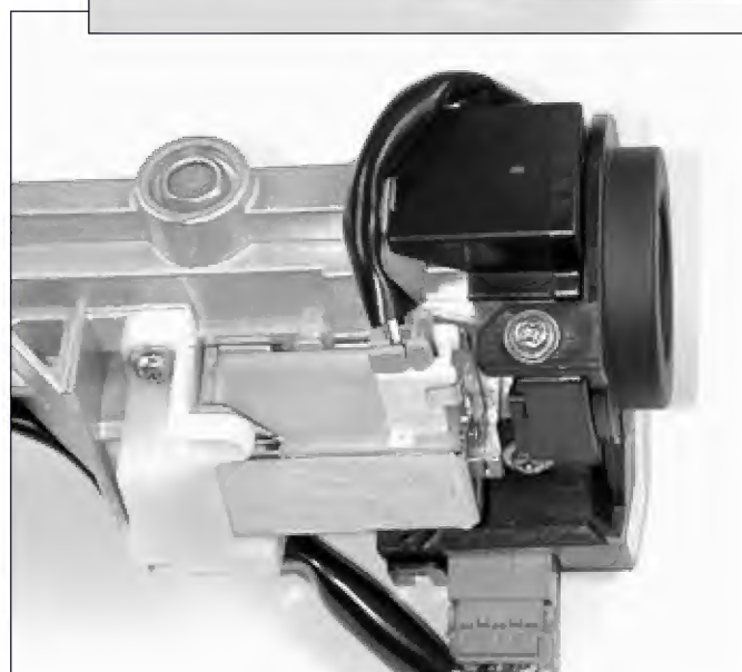
17. There is a Phillips-head screw on each side of the induction coil that must be removed.
