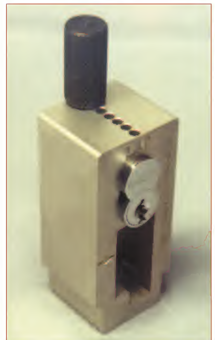
7. The tip of the Capping Tool is in the first chamber.
