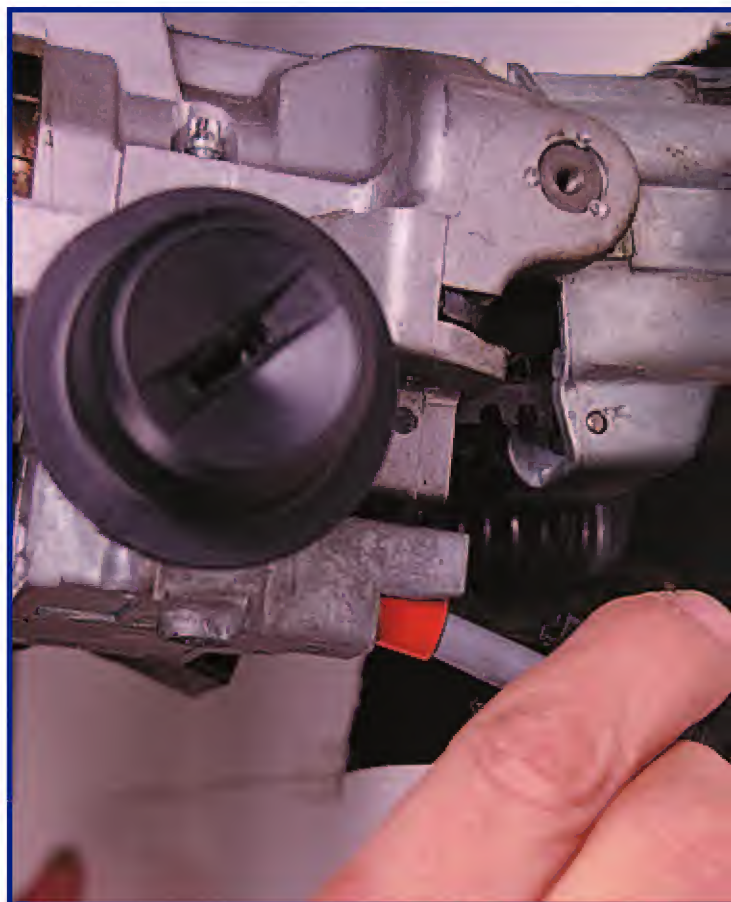
13. Pull the shift interlock cable out from the housing.
