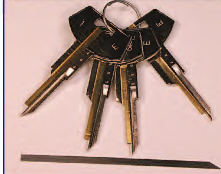
18. The AlphaCracker by Saber Tool Co. is a fast method for generating working keys for the Alpha Tech ignition.
