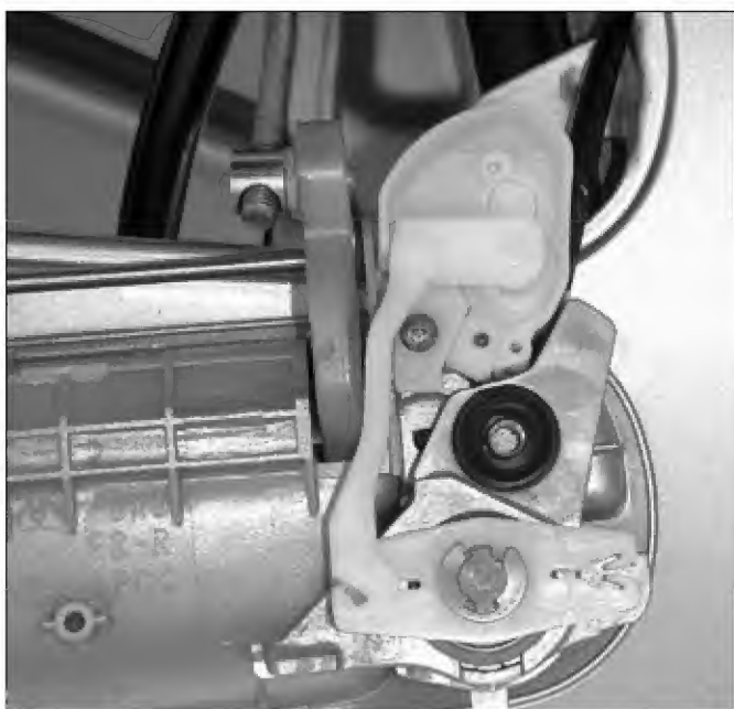
47. A view of the lock cylinder and handle assembly as it would be in the door.
