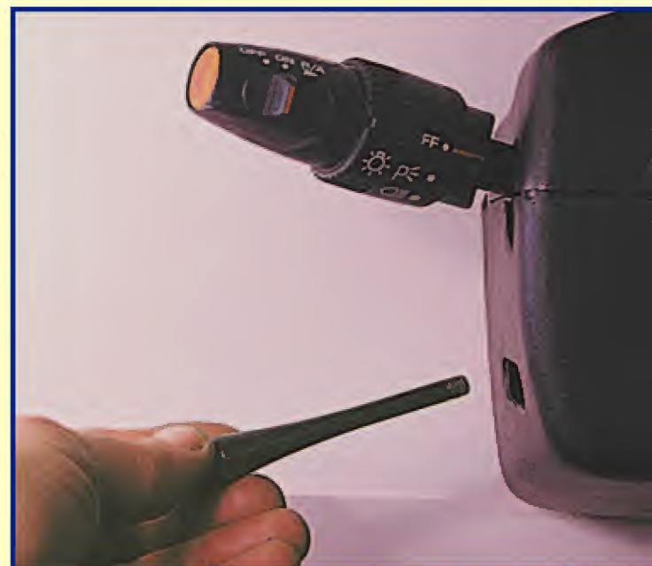
2. Remove the tilt lever arm.
