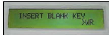
14. Insert the blank key into the key receptacle and press the "Wr" key.
