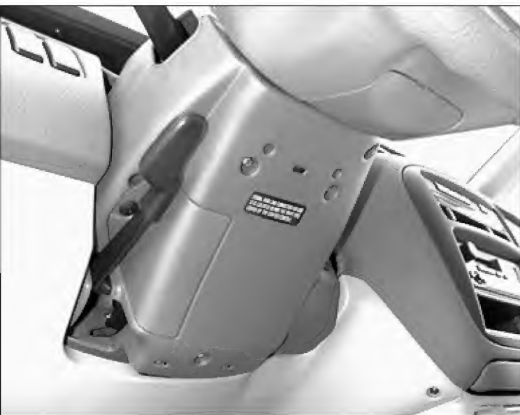
5. To remove the ignition lock you must first remove the plastic column shroud.
