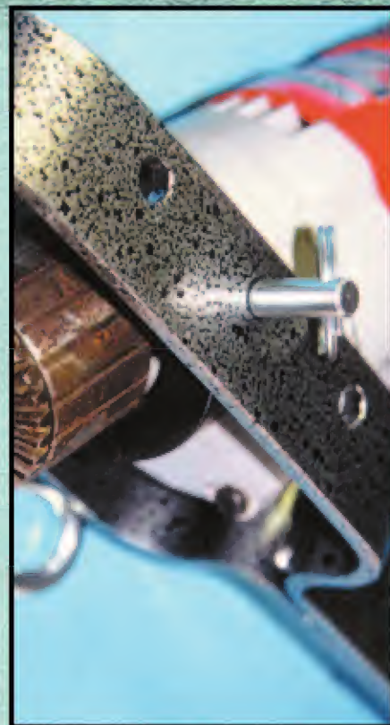
18. Quick release pins, one on each side. There are three positions to attach drill, depending on angle needed.
