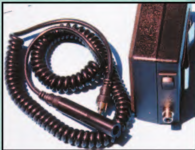
2. Battery operated light source and flexible cable comes with the unit. On-Off switch is located near cable plug.
