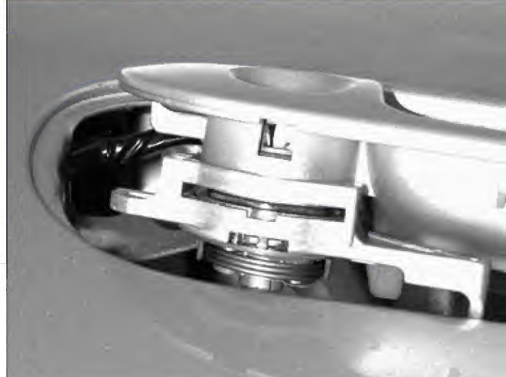
43. Remove the two 10mm bolts that hold on the outside door handle. You can now slide out the handle enough to gain access to the wire clip that holds on the cylinder to the handle. You must use a small flat blade screwdriver to get the clip out from around the lock cylinder.
