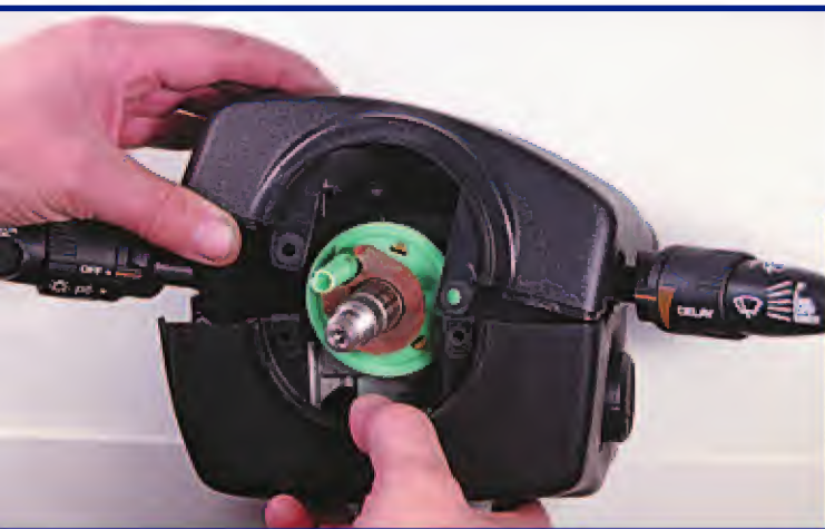
4. Lift the top shroud half up and out from the bottom shroud.
