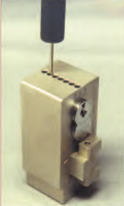
9. I have already ejected the cap, spring and pins from the first chamber.
