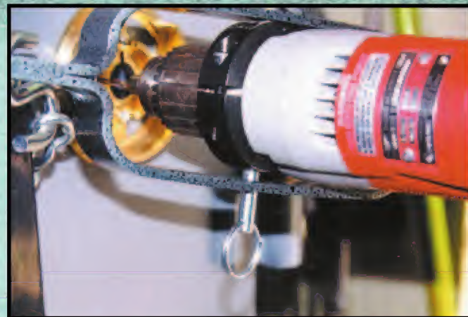
20. Rig in drilling position. Drill bit and attaching chain should be parallel.
