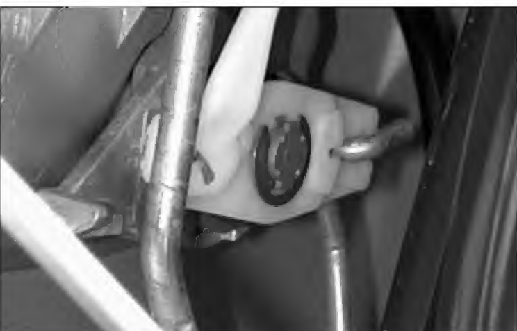
41. The best way to remove the lock cylinder is to take off the C-clip and slide off the tailpiece.
