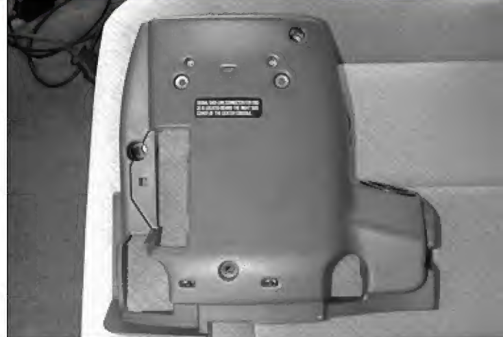
6. There are 6 Phillips-head screws to remove.
