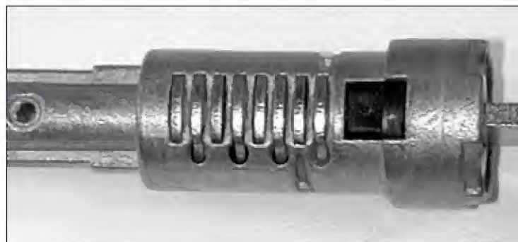
29. The ignition cylinder contains all 8 tumblers.
