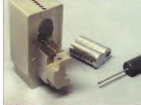
11. When the I-Core has been emptied, it should be removed from the fixture.
