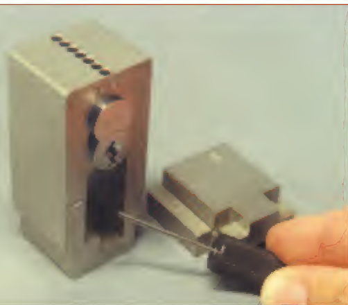
4. The I-Core should be pushed inward all the way until it stops.
