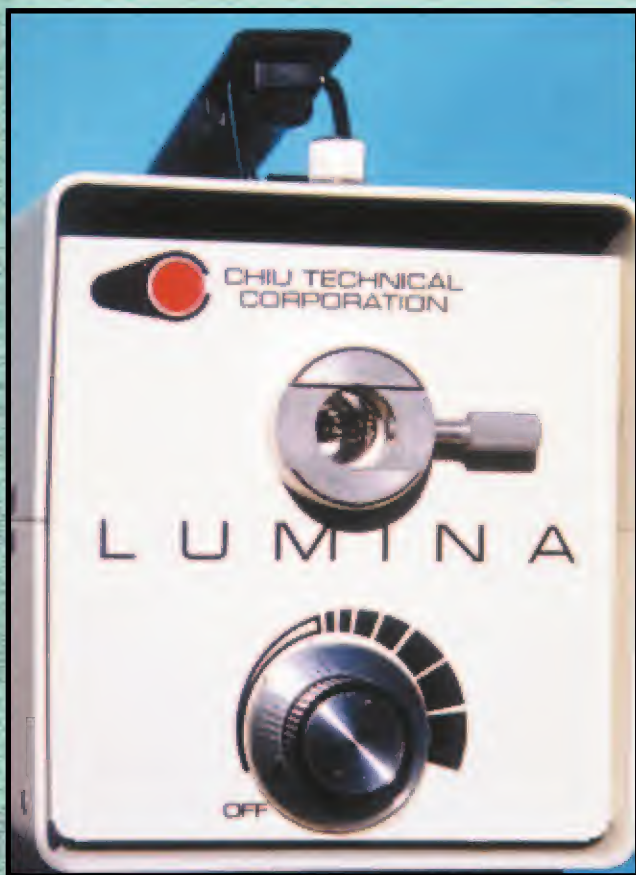
3. Additional light source with intensity dial at bottom and optic cable plug above.
