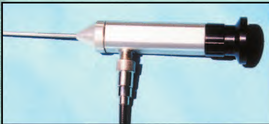
4. Optic cable plugged into borescope. This borescope has a focusing eyepiece for great viewing.
