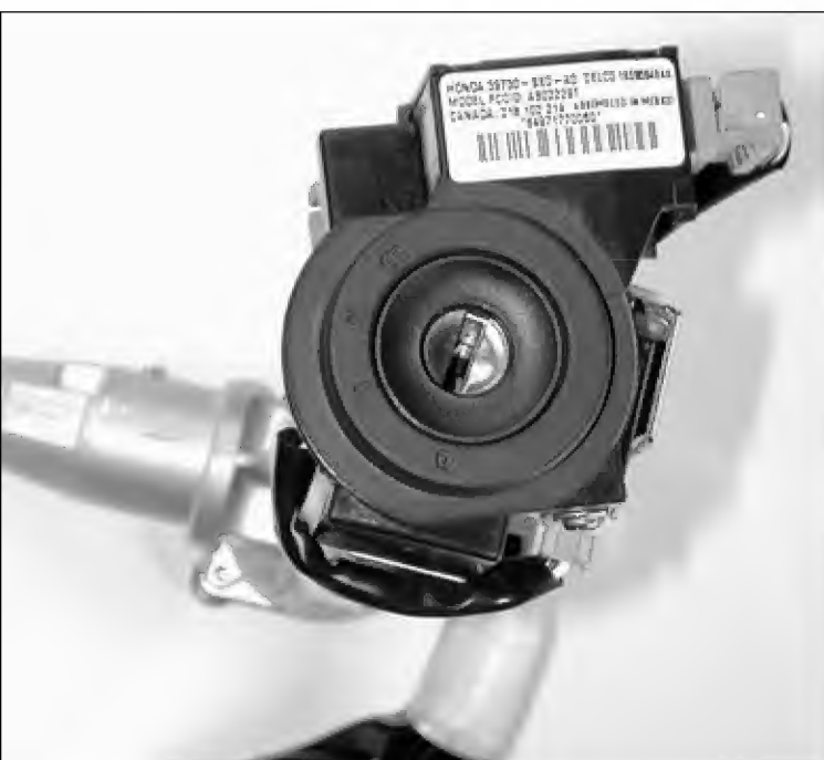
16. The transponder induction coil (antenna) mounts to the face of the lock housing.
