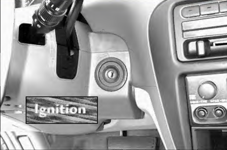
4. The ignition lock can be a real pain to get out. This van is equipped with a dealer only transponder system.
