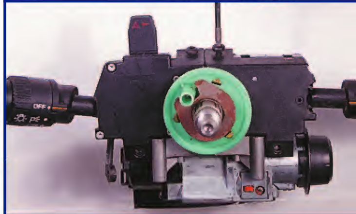
5. Remove the four screws holding the wash/wipe and turn signal switches.
