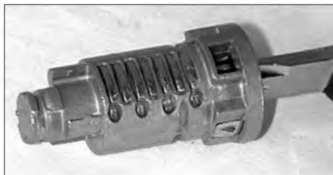
50. The cylinder plug contains 7 tumblers in positions 1 through 7.
