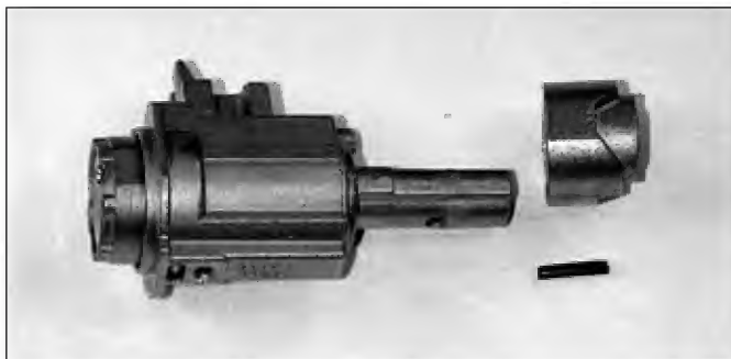
27. Once the roll pin is removed slide the cam off the back of the lock.
