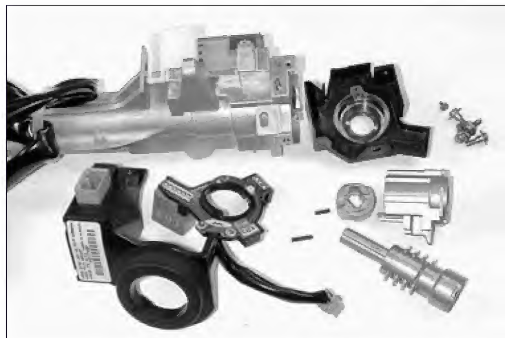
30. A view of the ignition lock cylinder disassembled.
