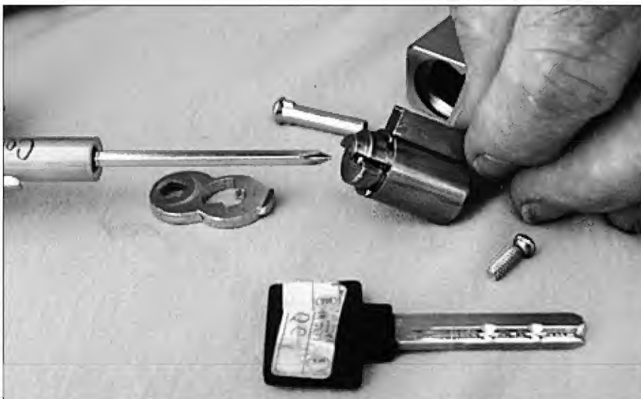
8. The screwdriver is pointing to the tailpiece of the lock.
