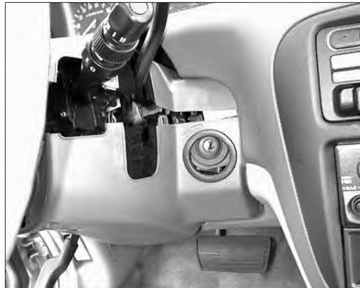
7. Once the screws are removed you can unsnap the plastic shroud. The shroud fits in the dash tightly and it may be necessary to remove the lower dash panel.
