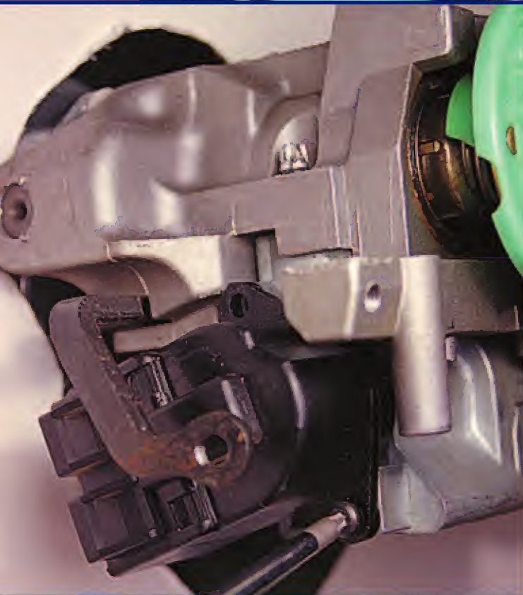
7. Remove the top and bottom screws that hold the ignition.
