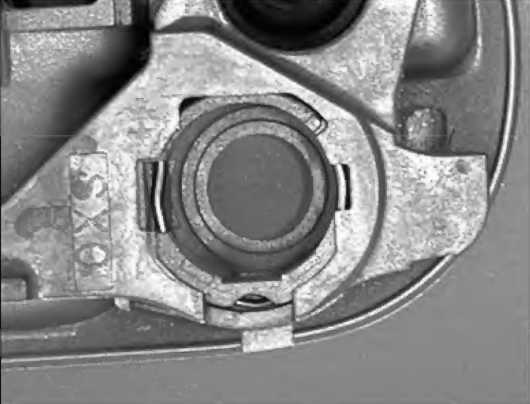
46. A view of the cylinder guard and the wire clip as it sits on the handle.
