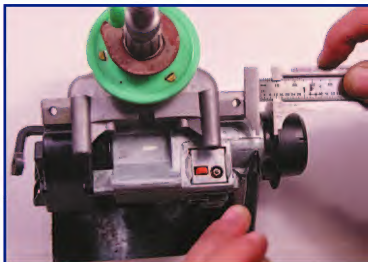
9. Carefully mark the outside of the housing for drilling.
