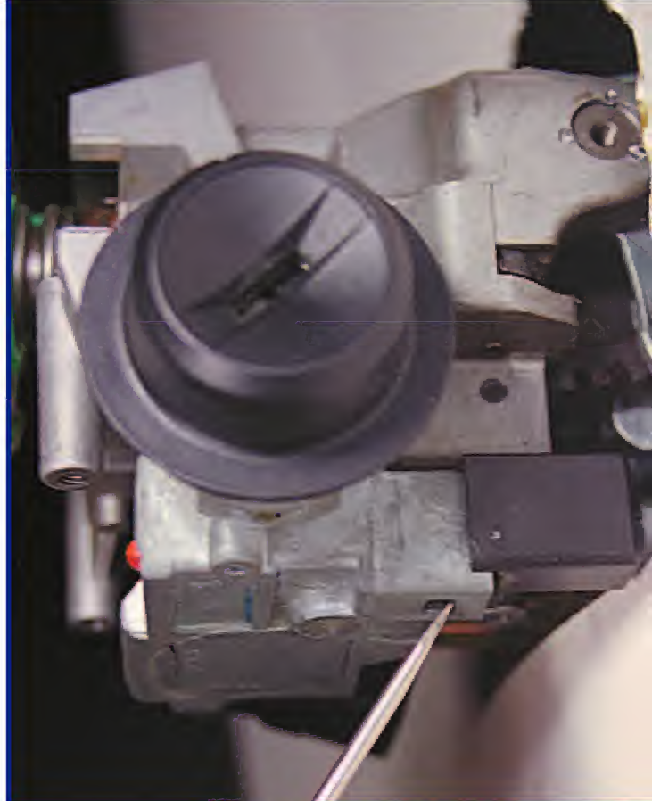
12. After turning the ignition to the ON position, use a small screwdriver to depress the shift interlock cable release tab.
