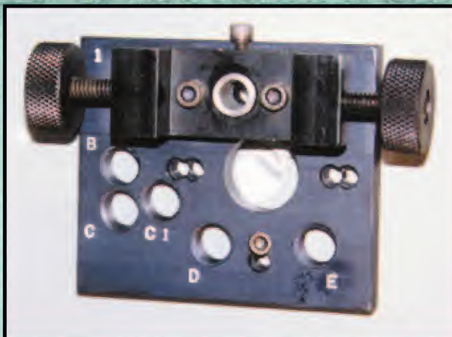
13. Drill base attaches with two hardened cap screws. Note removable bearing between screws.
