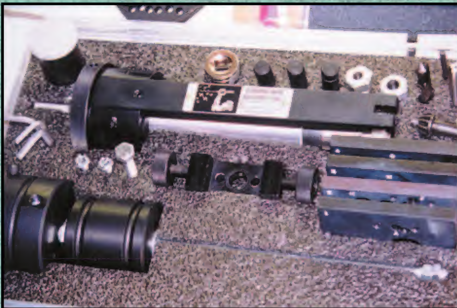
10. The new Mini-Rig with four basic templates and dial puller system.
