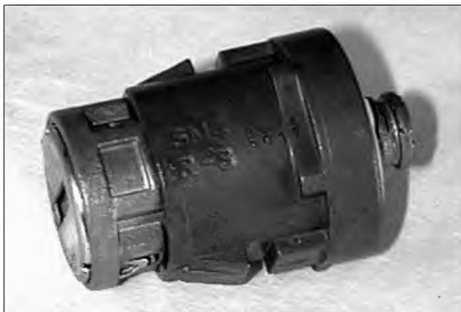
48. The door lock cylinder removed. There is a code stamped on the side of the lock. The code is the bottom 4 numbers. The code series runs from 5001-8442 with no prefix.
