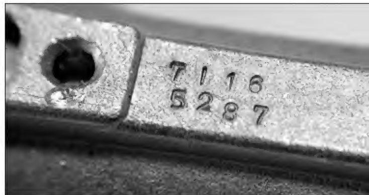
24. There is a code stamped on the lock cylinder. This is not a help since you have to do a lot of work to get the cylinder out.
