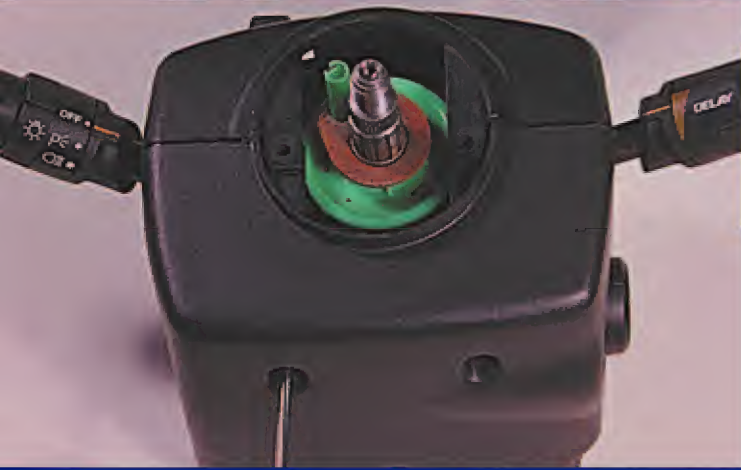
3. Use a T20 Torx driver to remove the shroud screws found at the bottom of the column.
