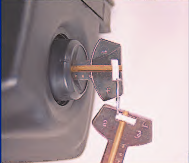
21. Push the key into the keyway until the first Position Index mark is aligned with the face of the ignition lock.
