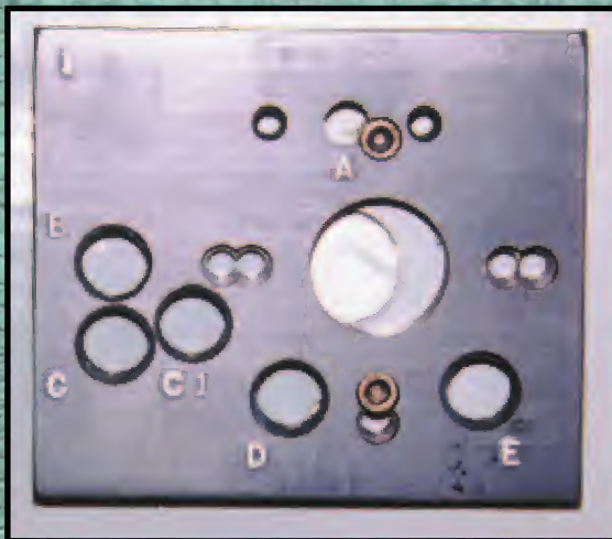
12. Basic template for S&G locks. "A" is the drop in position for a horizontal left mounted lock.
