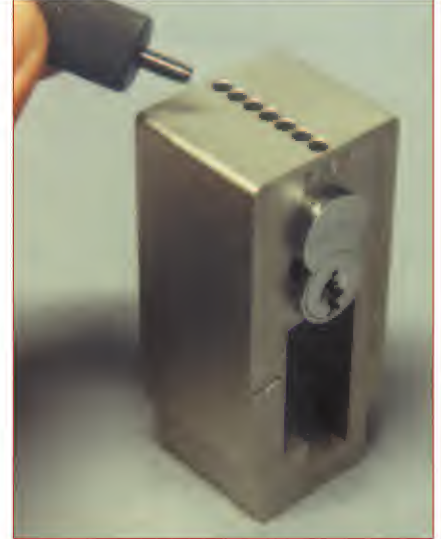
6. With the first chamber loaded the Evictor Tool is removed.
