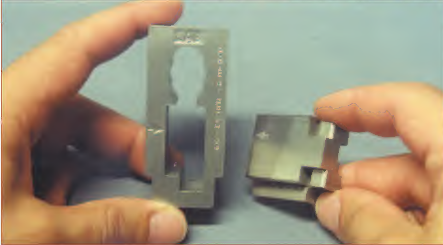
2. The part that holds the ejected pins and springs is called the "Code Book".
