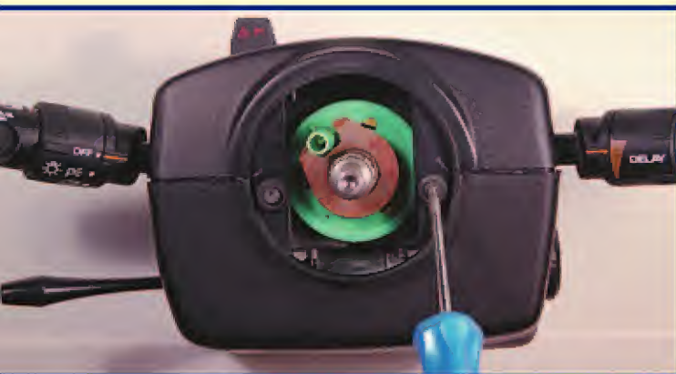
1. Hidden beneath the steering wheel are two T15 screws.
