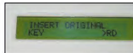
7. Display prompts you to INSERT ORIGINAL KEY (and press)-RD.
