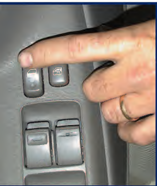
3. Cycle through Lock/Unlock using electronic lock button.
