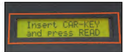
21. Insert the customer's key into the key receptacle, and press the RED "read" button.
