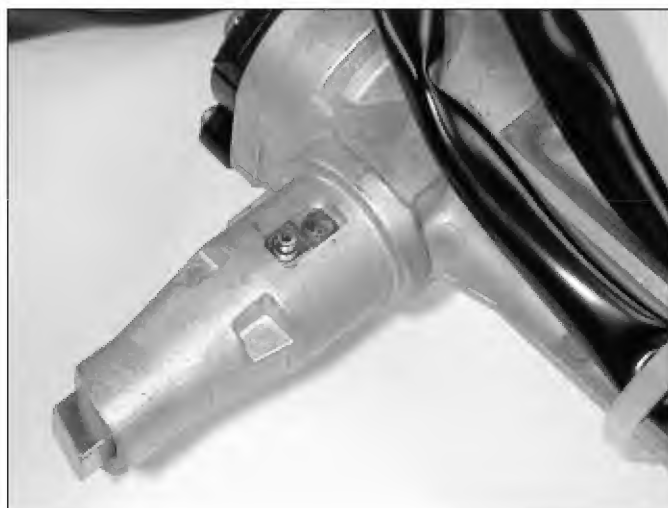
15. A view of the active retainer. The key must be turned to the ON position to depress the retainer.
