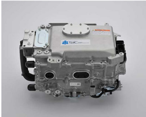
Fig. 20. Toyota SiC power control unit [81].
