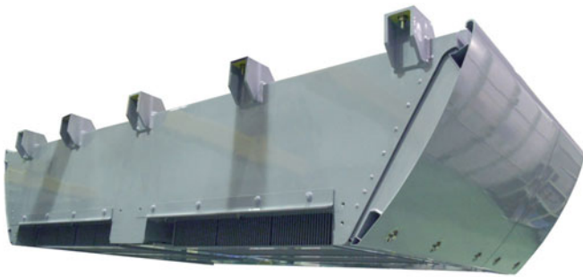
Fig. 19. Mitsubishi all-SiC modules based traction converter [77].
