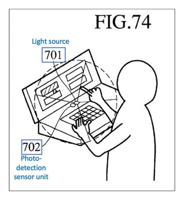
*Id.* at Figure 74 (annotated to indicate light source 701 and photo-detection sensor unit 702).
