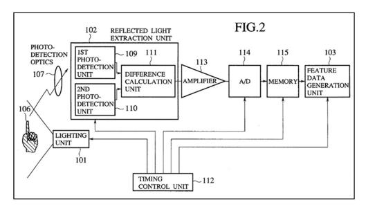
*Id.* at Fig. 2. A timing control unit is used to turn lighting unit 101 on (i.e., illuminating the target object) when the first camera unit is active and off when the second camera unit is active. *Id.* at 11:20-32. The result of this light control is the first camera unit captures an image of the target object illuminated by both natural light and the lighting unit 101 and the second camera unit captures an image of the
