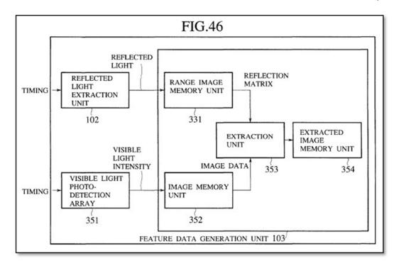
*Id.* at Fig. 46. Using this arrangement, the fifth embodiment processes the output of two-sensor structure 102 to identify an outline of the subject and subtracts everything outside this outline from the image captured by the visible light sensor 351. *Id.* at 39:24-60.
