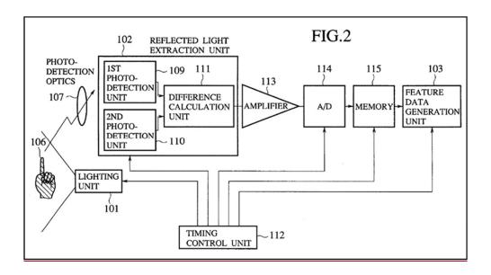
*Id.* at Fig. 2. A timing control unit is used to turn lighting unit 101 on (i.e., illuminating the target object) when the first camera unit is active and off when the second camera unit is active. *Id.* at 11:20-32. The result of this light control is the
