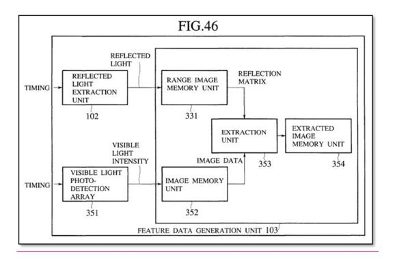
Id. at Fig. 46. Using this arrangement, the fifth embodiment processes the output of two-sensor structure 102 to identify an outline of the subject and subtracts everything outside this outline from the image captured by the visible light sensor 351. Id. at 39:24-60. In doing so, the fifth embodiment arrives at image information that contains only the subject without any background image information and uses much less data as a result of removing the extraneous image information. Id. at 40:32-35
