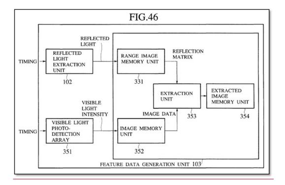
*Id.* at Fig. 46. Using this arrangement, the fifth embodiment processes the output of two-sensor structure 102 to identify an outline of the subject and subtracts everything outside this outline from the image captured by the visible light sensor 351. *Id.* at 39:24-60.
