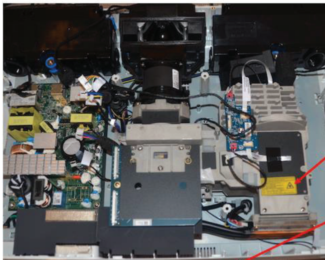
Open top of projector showing laser light source and warning label
