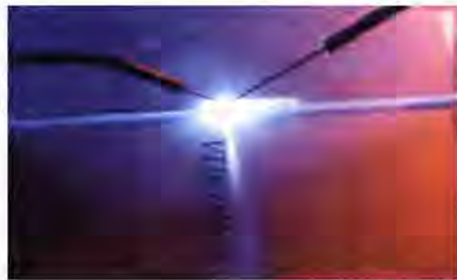
Figure 6 Laser diode operating under pulsed current injection of 1.4 A at room temperature 47 (courtesy of S. Nakamura, Nichia).
