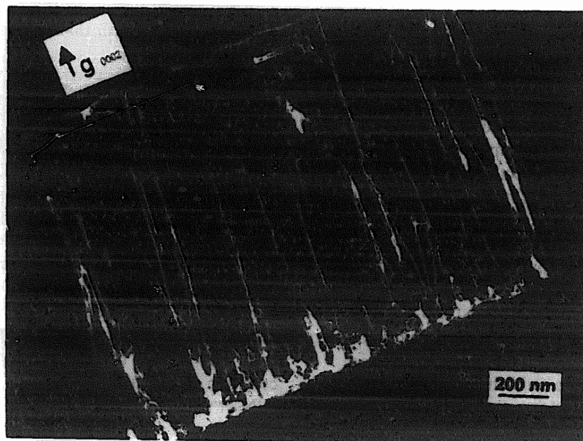
Fig. 1. Transmission electron micrograph of a GaN film grown by MBE on sapphire without the use of a buffer layer. Note the high density of misfit dislocations and other structural defects at the substrate interface. A high density of threading dislocations also persists further away from the substrate.
